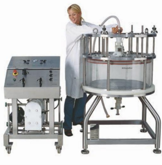
Fig 3. Packing Chromaflow columns with the dedicated packing station is convenient and simple.
