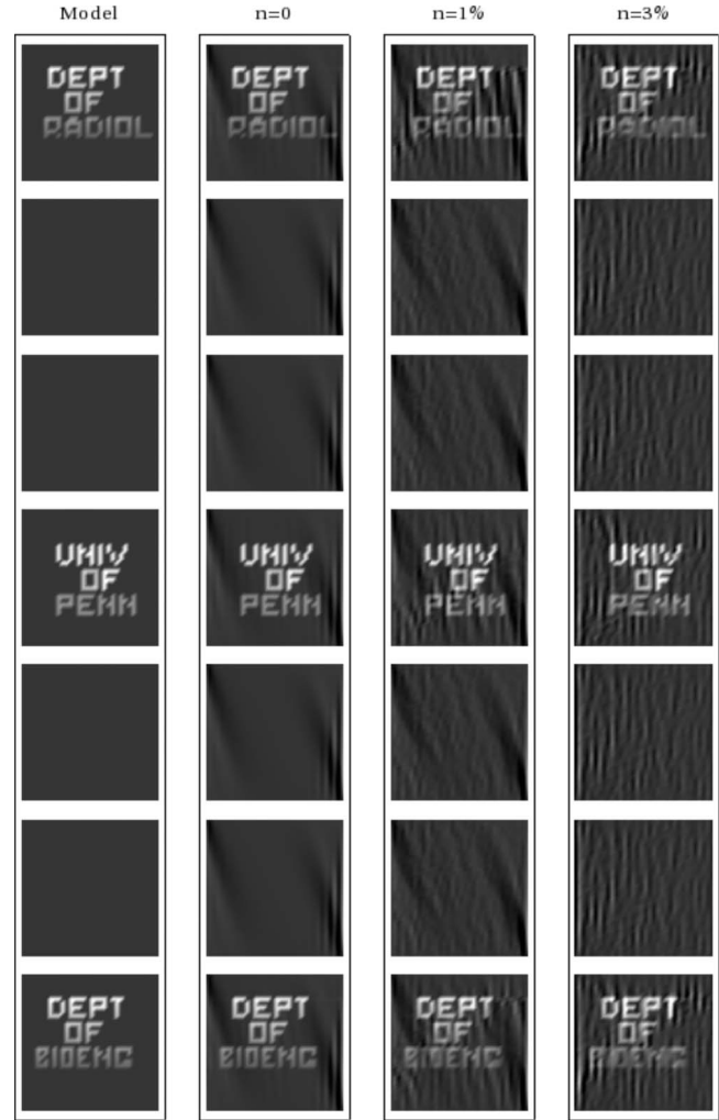
FIG. 5. Image reconstruction for a slab with \mu_s=0.04h^{-1} and various noise levels n . The absorbing inhomogeneities are placed in the slices x=6h , x=13h , and x=20h and the rows show the slices x=6h , 7h , 12h , 13h , 14h , 19h , and 20h . The same color scale is used for all slices, with the target maximum (white) corresponding to \mu_t=0.24h^{-1} and the minimum to \mu_t=0 .
