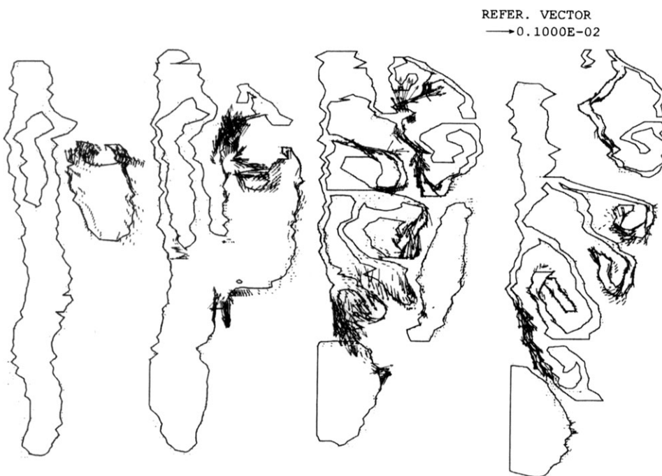
Figure 10 Vector plots of the inspiratory rat nasal cavity uptake of the odorant octane (very insoluble in mucus) for a half nasal flow rate of 504 ml/min. Note the mostly lateral deposition compared to the more soluble l -carvone shown in Figure 9. Reference vector represents magnitude of 1 \times 10^{-3} g octane deposited/cm 2 ·s. Flow is out of plane of paper.
