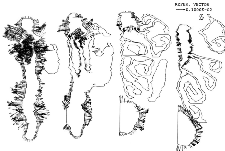
Figure 9 Vector plots of inspiratory uptake of the odorant l -carvone (moderately soluble in mucus) on four rat nasal cavity cross sections (Yang numbers 163, 176, 200, 226) left to right, anterior to posterior. Half nasal inspiratory flow rate is 504 ml/min. Reference vector represents 1 \times 10^{-3} g l -carvone deposited/cm 2 ·s. Note medially located deposition. Flow is out of plane of paper.
