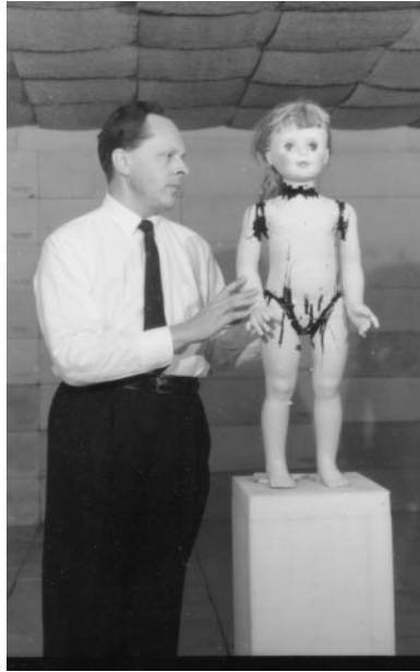
Figure 9 Schwan with model of human body used for RF dosimetric studies. The model is filled with tissue-equivalent liquids and exposed to RF energy in a microwave-anechoic chamber that Schwan had constructed in his laboratory. Photograph from ca. 1963.
