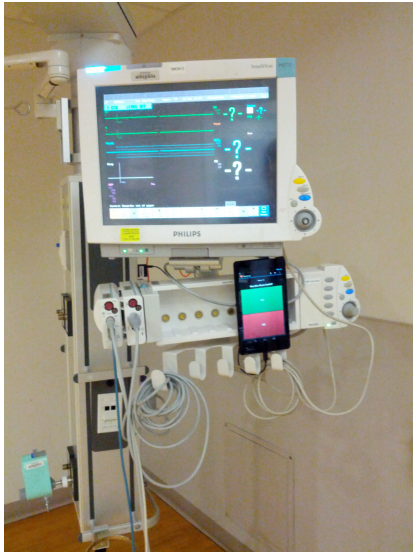
Fig. 1. A bedside monitor at Penn Presbyterian Medical Center in an (empty) patient room. An annotation tablet, with our application running, is mounted below the lower right side of the screen (see Section IV-A).
