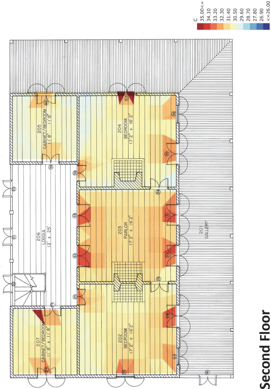
Figure 35. Indoor operative temperatures of the Pitot House on June 21st at noon. Drawing underlay sourced from HABS.
