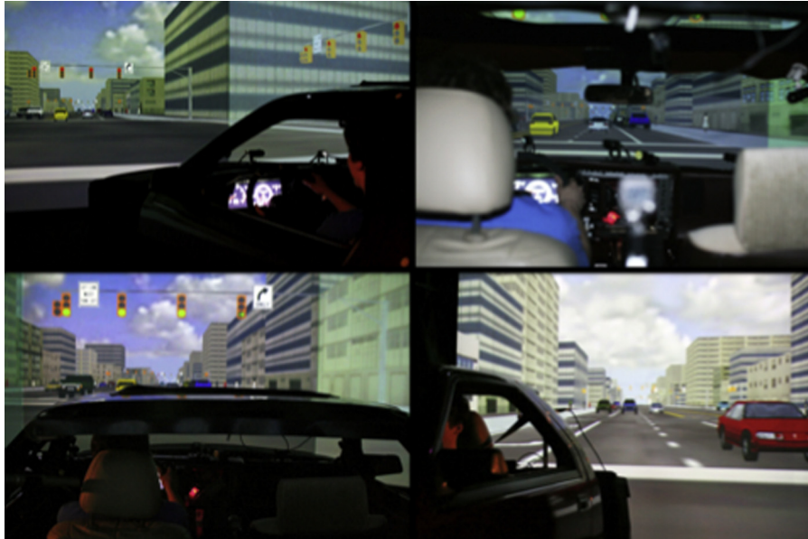
Figure 2. Driving simulator. During the driving session, participants drove in a fixed-base, partial cab driving simulator.
