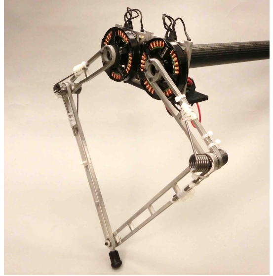
Fig. 2: The control behaviors were demonstrated on a hopping robot fixed to a boom, constraining the body in all degrees of freedom but the horizontal and the vertical.
