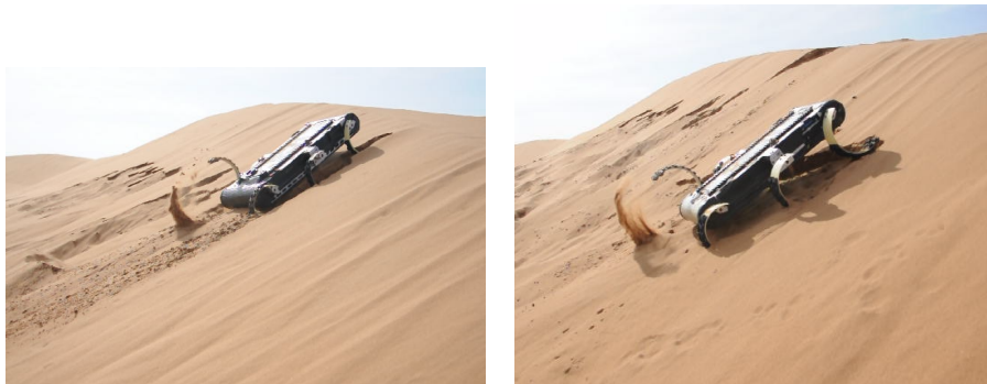
(a) Successful ascent of a 30-degree dry slope by the thin-legged robot performing a fast crawl.
