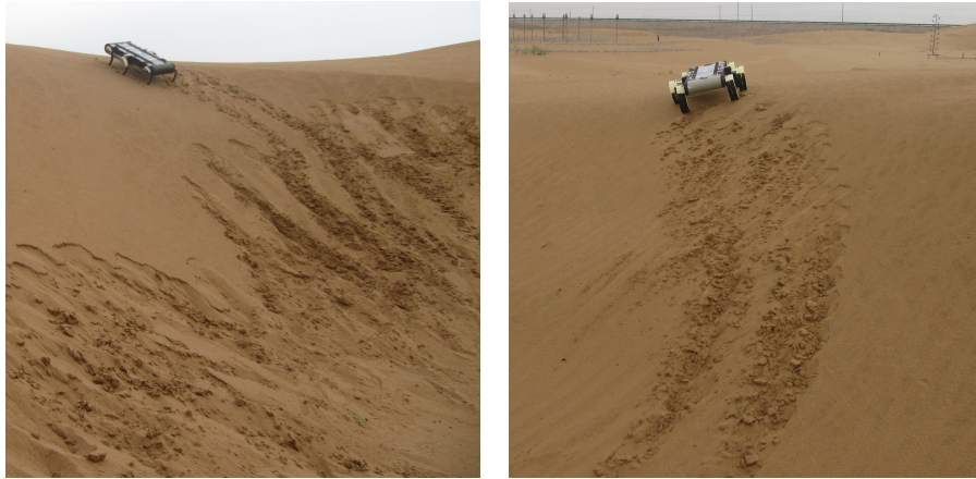
(a) Natural yaw during vertical ascent with thin legs. (b) Natural yaw during vertical ascent with fat legs.
