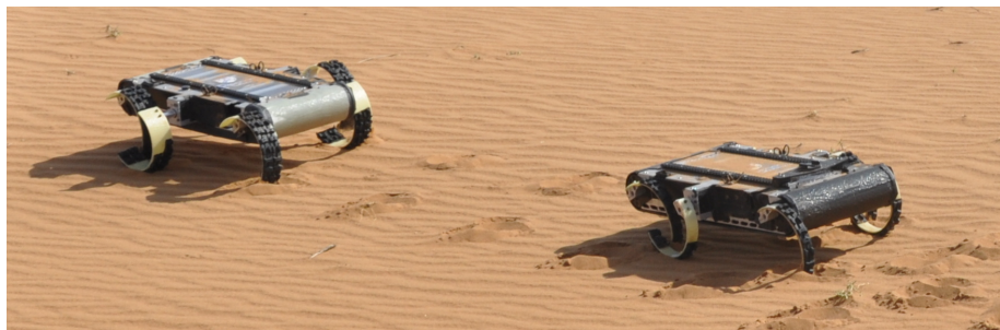
Figure 8: Specific resistance experiment in which the two robots walked together for 30 minutes over the same territory.
