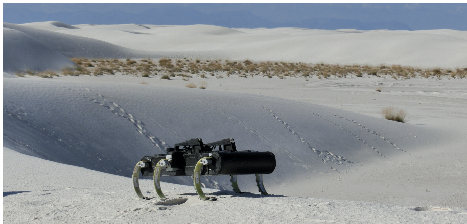
(c) D-RHex on a dune crest at the White Sands national monument. Future experiments could involve taking measurements while traversing dune crests during wind events of interest.
