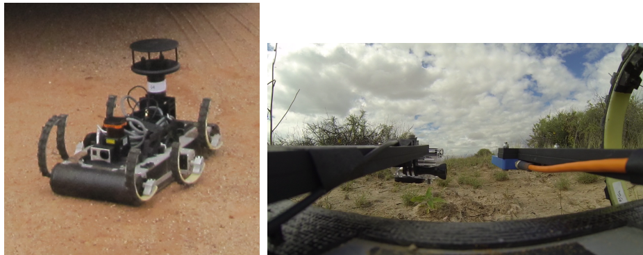
(a) D-RHex with forward facing camera (b) A sample image taken by the forward facing GoPro camera
