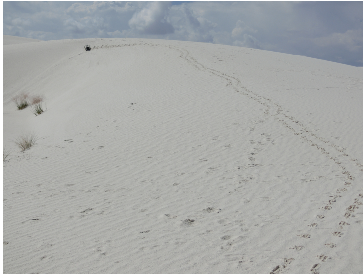
(a) Dune crest traversal failure. The tracks show the robot's path as it traveled along the dune crest. Near the top of the dune the human operator mistakenly veered the robot onto the slip face and it was unable to ascend directly back to the top.
