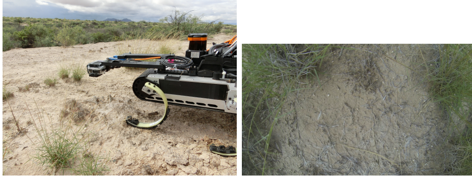
(a) D-RHex with downward facing camera on the left arm (b) A sample image taken by the downward-facing GoPro camera
