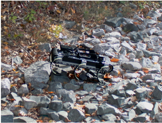
FIGURE 6. X-RHex performing a reactive stand on rocks.
