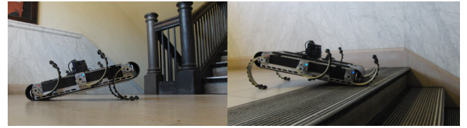
FIGURE 8. Robot performing two pitching sensor sweeps with a planar laser scanner: (Left) upward ( \phi > 0 ) to scan a staircase, (Right) downward ( \phi < 0 ) to check for a cliff.
