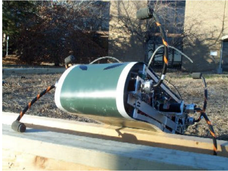
Figure 1: The RHex robot running at a body length (~50cm) per second over rough terrain.
