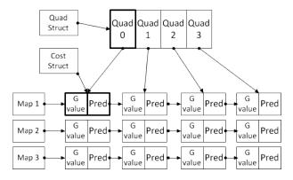
Fig. 2. Quad struct and cost struct layout. For each quad, there are as many cost structs as goals in the map.
