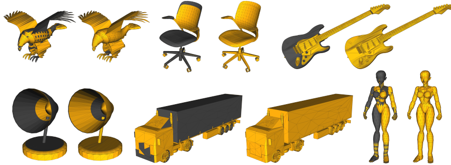
Figure 6. Results of our method. In each pair, the original facet orientations and the facet orientations corrected by our method are shown on the left and on the right, respectively.
