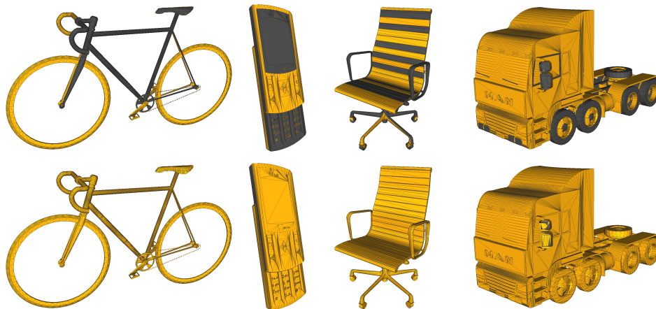
Figure 1. A few examples of meshes from the SHREC'10 Generic 3D Warehouse dataset [Vanamali et al. 2010] with incorrect facet orientations (top row), and the results of our automatic correction method (bottom row).
