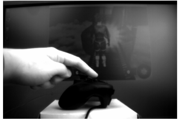
Figure 13: A high speed camera was used for accurate latency measurements. We determined the time between the push of the gamepad button and the character’s response.
