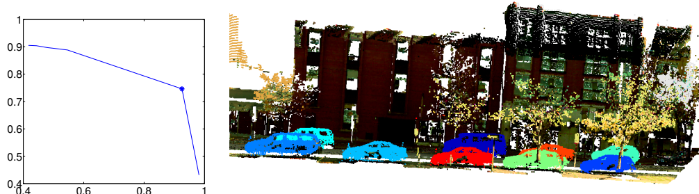
Figure 4.6: Left: The precision-recall curve for car detection on 200 million points containing 1221 cars. (Precision is the x-axis and recall the y-axis.) Right: Screenshot of detected cars. Cars are in random colors and the background in original colors.
