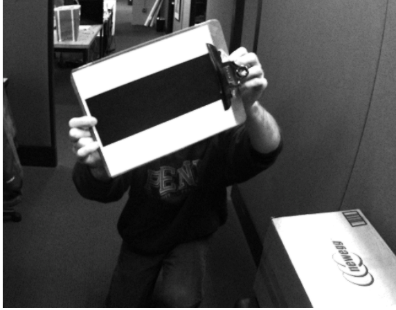
Figure 2.2: A single camera frame from the calibration data set showing the calibration object. The object consists of a black line on a white sheet of paper. We detect the white-to-black transition looking from the top of the image.
