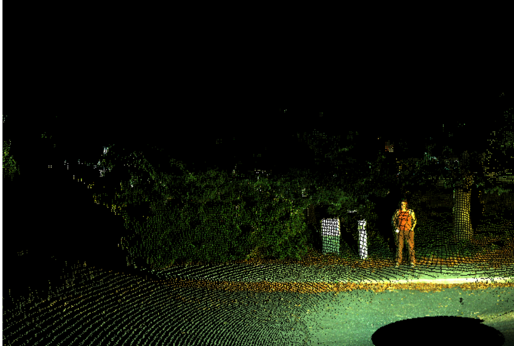
Figure 2.7: A LiDAR scan colored using camera pixels.
