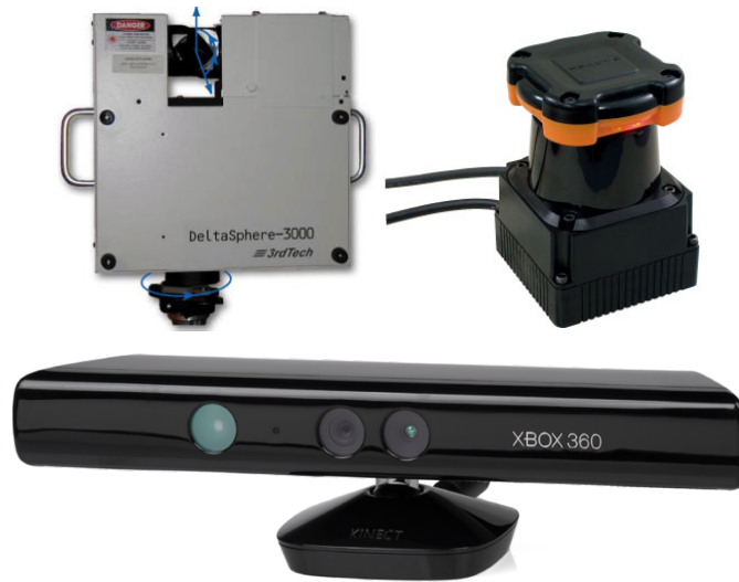
Figure 1.1: Three laser scanners are shown. Clockwise from top left: the 3rdTech Deltasphere, the Hokuyo UTM-30LX, and the Microsoft Kinect sensor.
