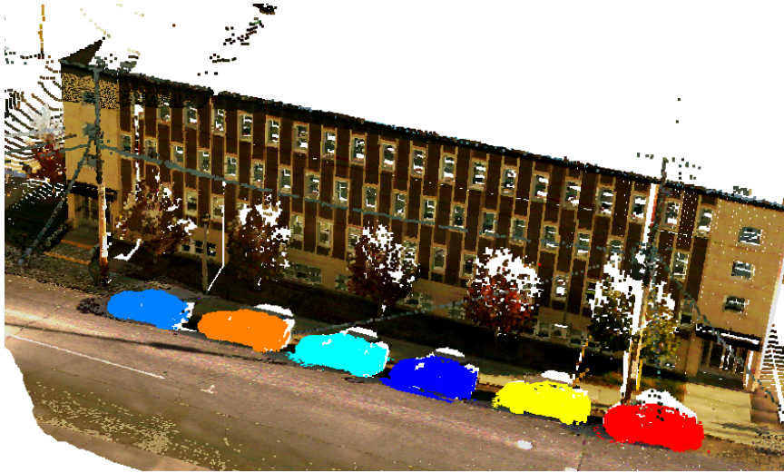
Figure 4.1: Cars detection results from real LiDAR data. Cars have been colored randomly.
