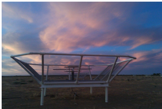
Figure 3.2: Photograph of a PAPER element, showing the groundscreen and the sleeved dipole.
