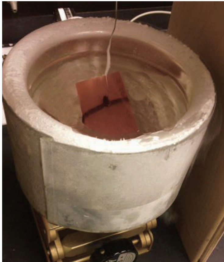
Figure 4.2.1 The experimental setup of liquid nitrogen porosimetry test 25
