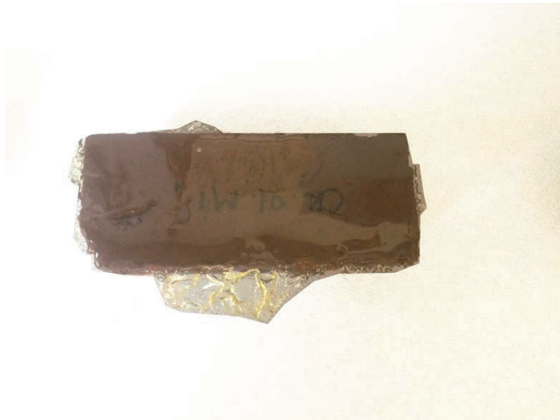
Figure 6.3.5 CR brick immersed in Tung oil for over 24 hours
