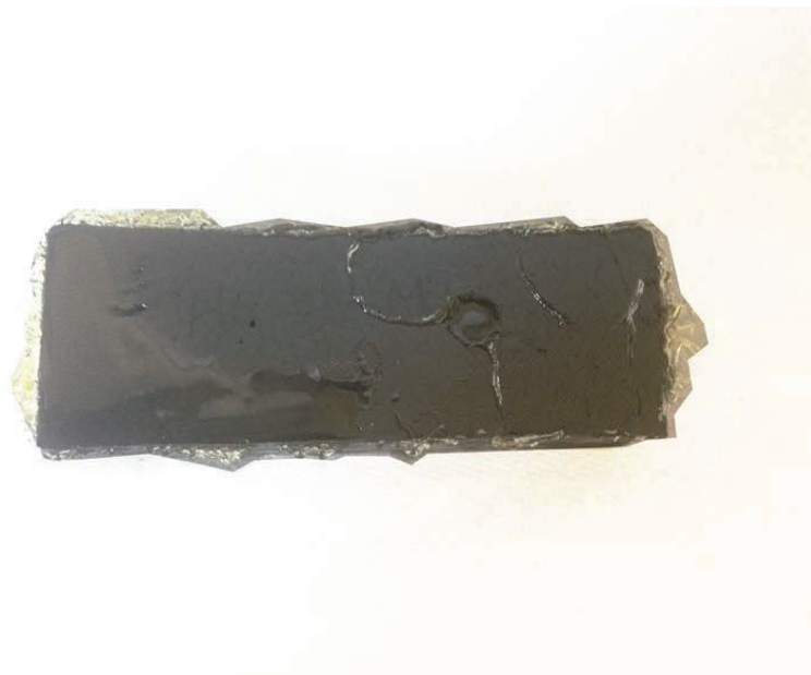
Figure 6.3.3 HG brick immersed in Tung oil for over 24 hours
