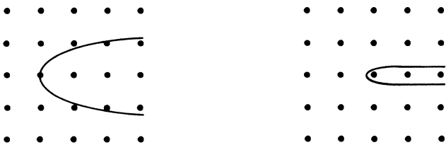
FIG. 5. Ellipsoids which are (left) and which are not (right) consistent with the lattice cut-off to serve as models for aggregates.
