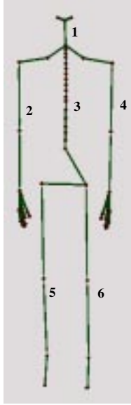
Figure 3.4: Sets of joint chains defined in the human model
