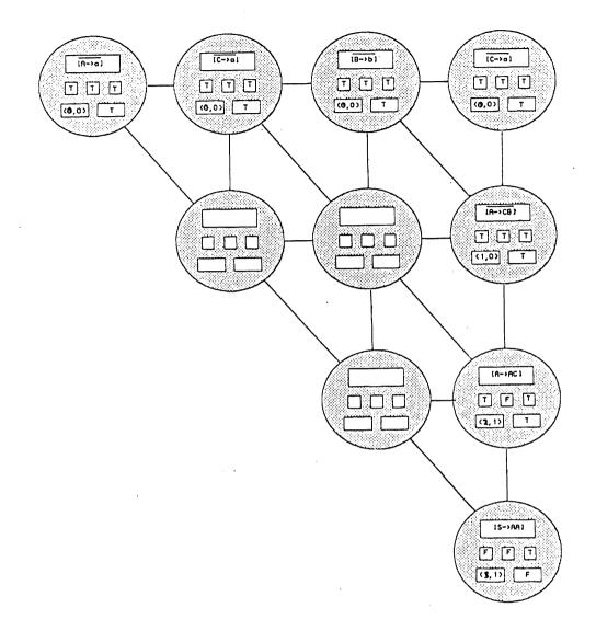
Figure 5.3. Register contents of the Q-array after the update step of stage 1.
