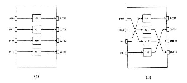
Figure 4.4. Updating the  $r_{pq}$  registers of processor P(i,j) for the case (a)  $2i \neq j$  and (b) 2i = j.
