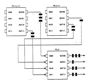
Figure 4.3. The  $IN_{pq}$  and  $OUT_{pq}$  terminals of a P-processor and their interconnections.
