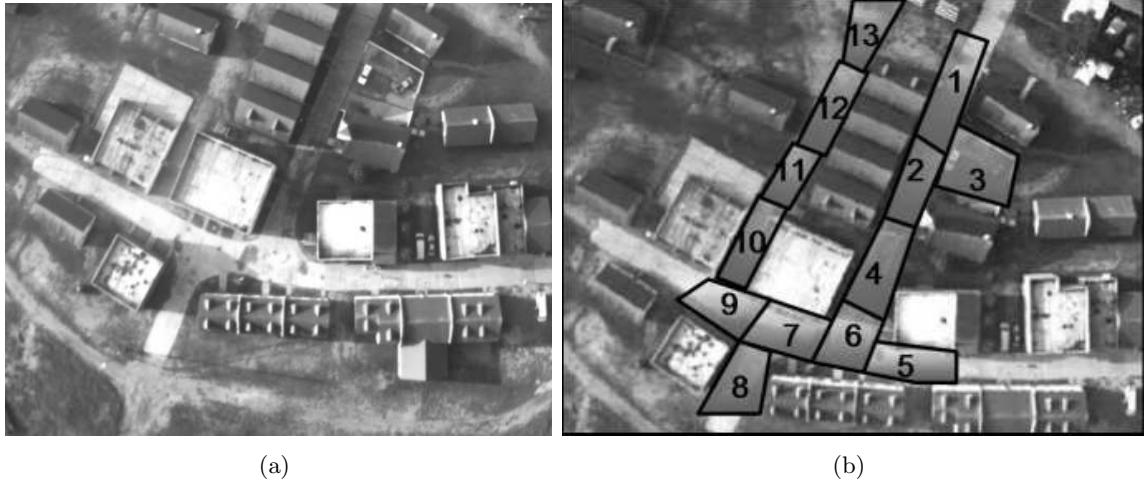
Figure 3: (a) A typical surveillance picture from our fixed wing UAV taken at an altitude of 150 m. The area shown is approximately 90 \text{ m} \times 120 \text{ m} . (b) A manual cell decomposition of the free configuration space for the site shown in Figure 3(a).
