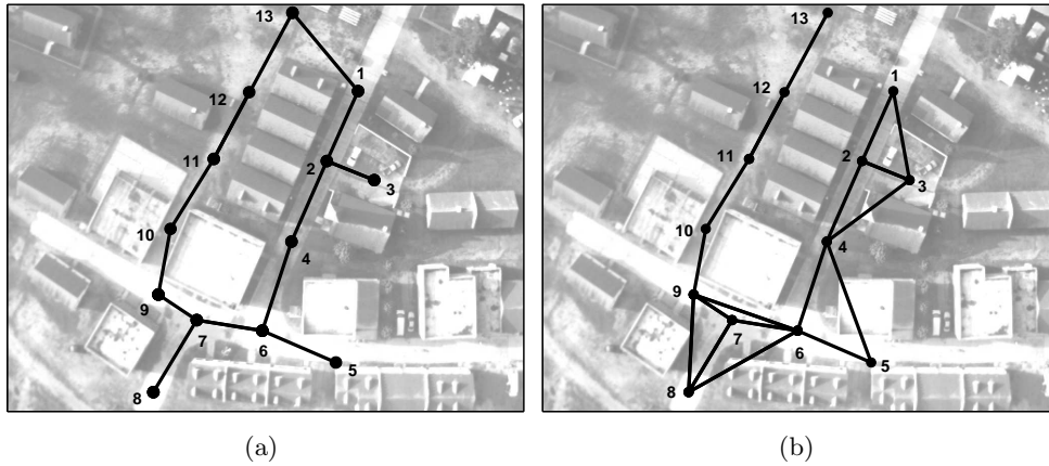
Figure 8: (a) Roadmap graph used for the site shown in Figure 3(a). (b) Radiomap graph for the site shown in Figure 3(a).
