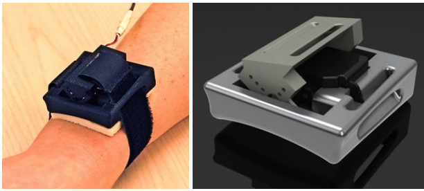
Figure 7: Left: The squeezer attached to a user's wrist. Right: A SolidWorks rendering of its mechanical design.
