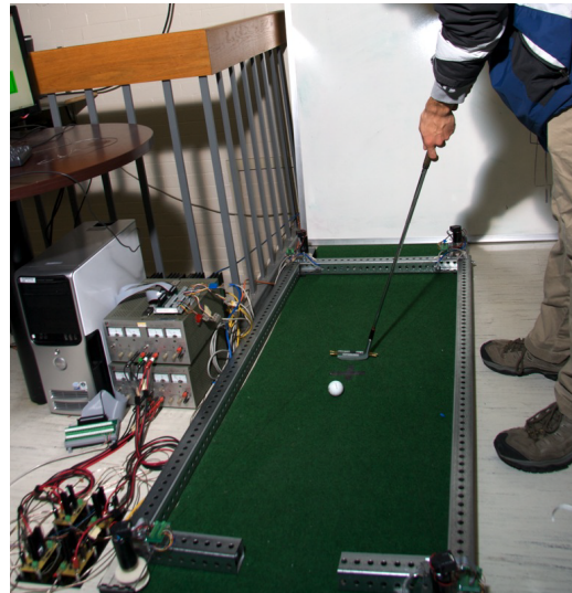
Figure 1: The planar four-cable haptic putting system. Though difficult to see, the cables extend from the edges of the putter head to the motors located in the four corners of the rectangular metal frame.
