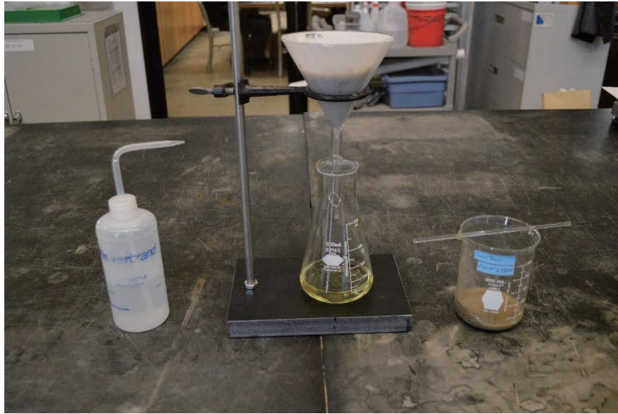
Figure 5.8 Setup of the fines separation (Author 2015).
