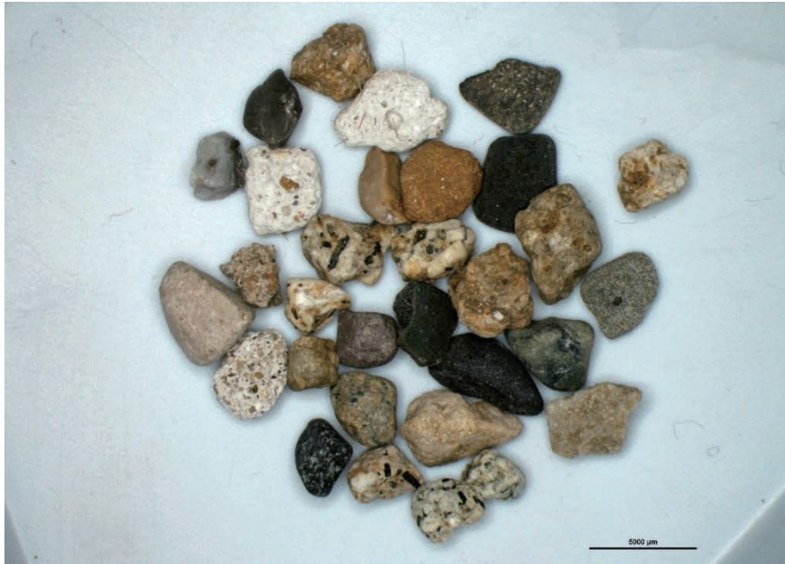
Figure B.1 Aggregate from sieve #8 (Author 2015).
