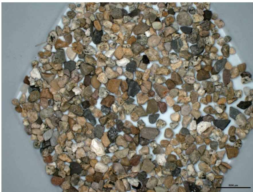
Figure B.2 Aggregate from sieve #16 (Author 2015).
