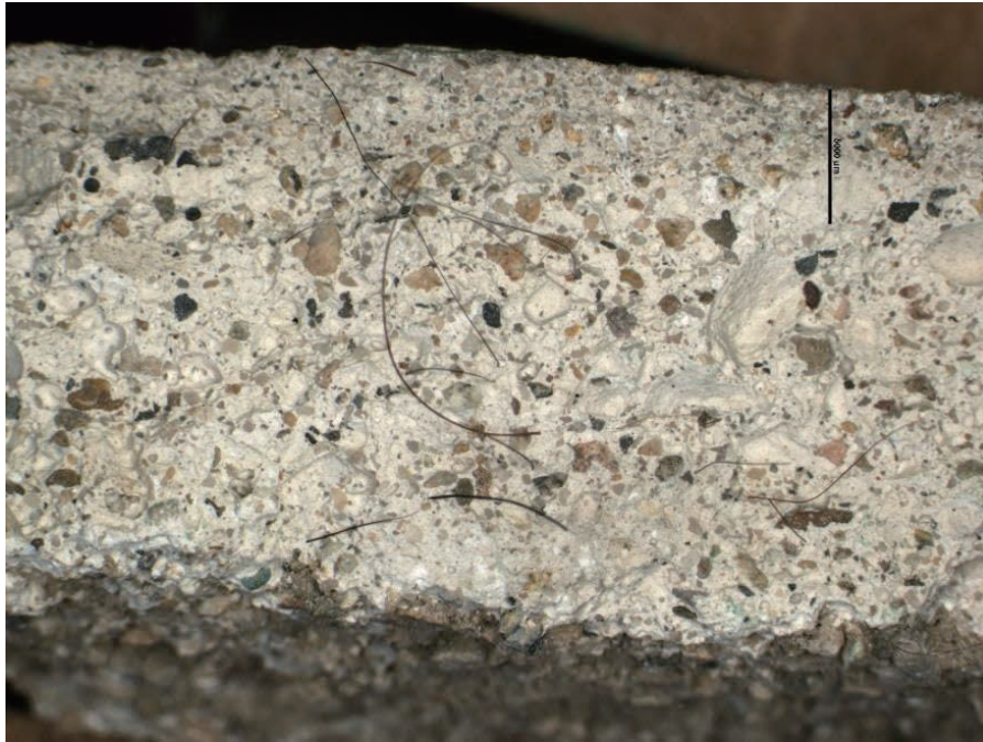
Figure 6.9 Photograph of bulk sample at 12.5x zoom showing multiple layers, colored aggregate and black hair (Author 2015).
