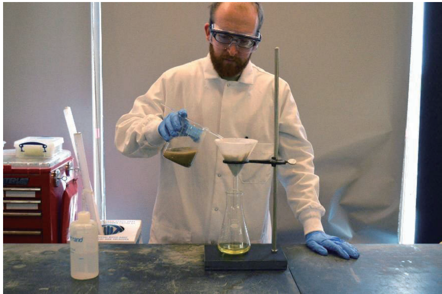
Figure 5.9 Author filtering suspended fines (Shuyi Yin 2015).
