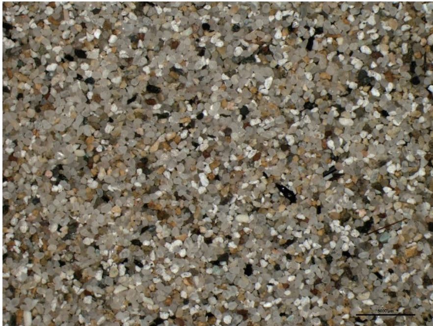
Figure B.5 Aggregate from sieve #100 (Author 2015).
