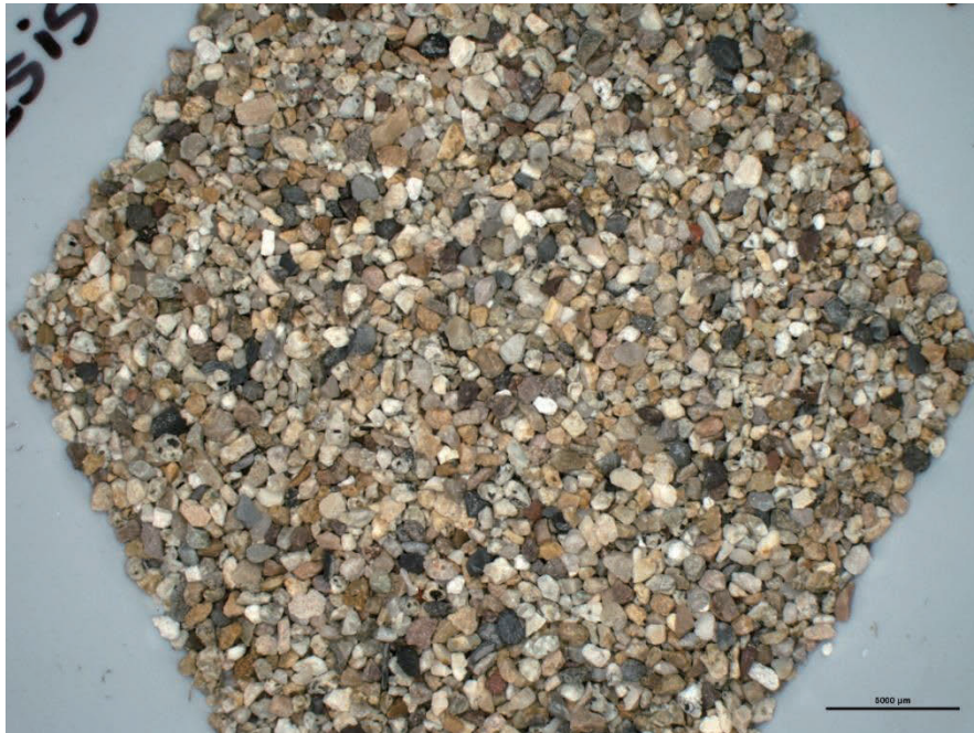
Figure B.3 Aggregate from sieve #30 (Author 2015).
