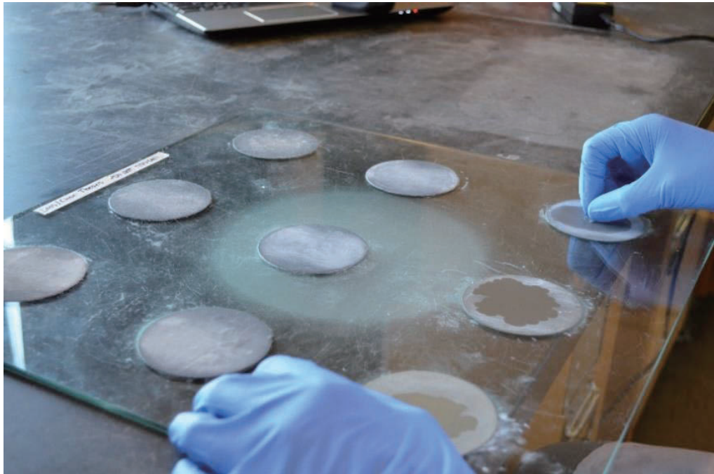
Figure 5.2 Detail view of polishing (Jocelyn Chan 2015).
