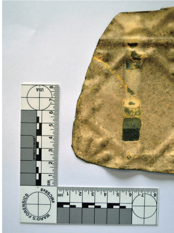
Figure 6.8 Exposure of pressed metal ceiling finishes stratigraphy (Author 2015).
