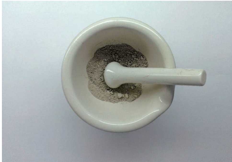
Figure 5.5 Crushed plaster sample (Author 2015).
