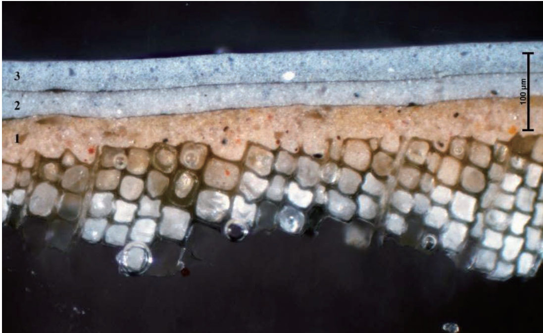
Figure 6.1 Sample MTT 04 showing its original cream orange finish (Author 2015).
