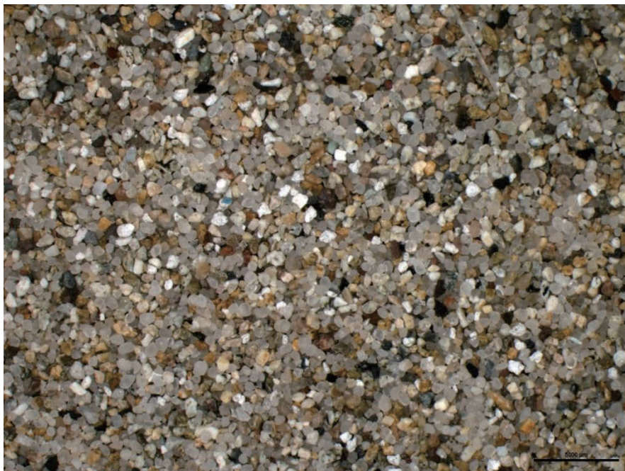
Figure B.4 Aggregate from sieve #50 (Author 2015).
