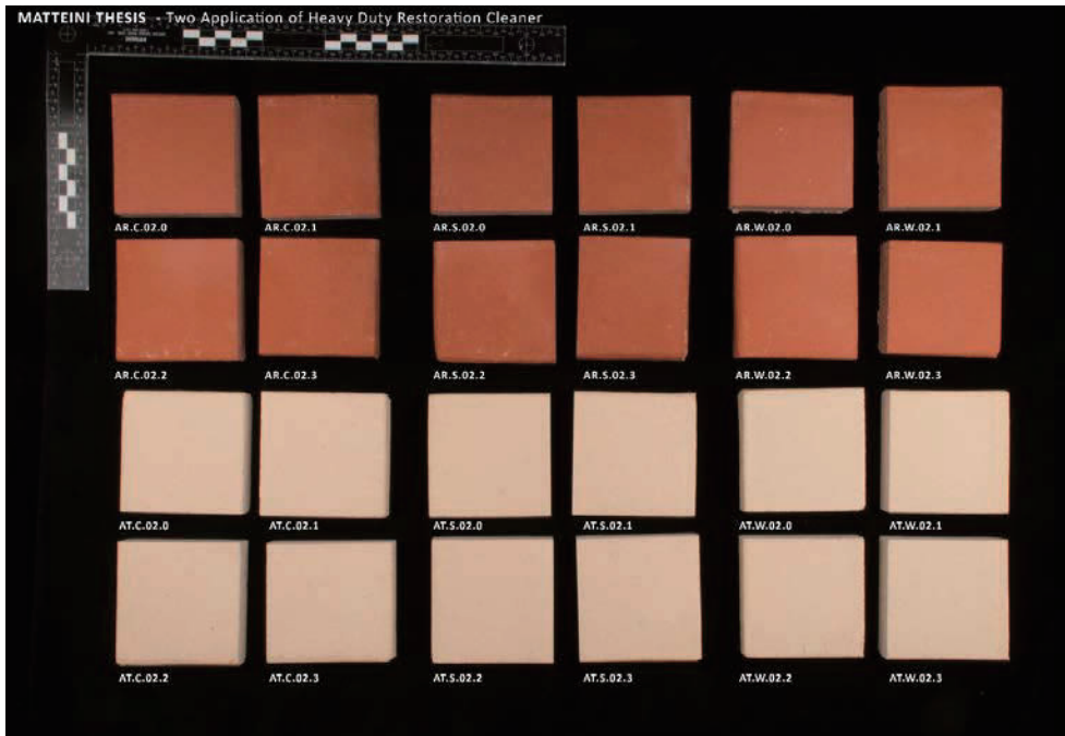
Figure 15: Sample set treated with two application of ProSoCo Heavy Duty Restoration Cleaner
