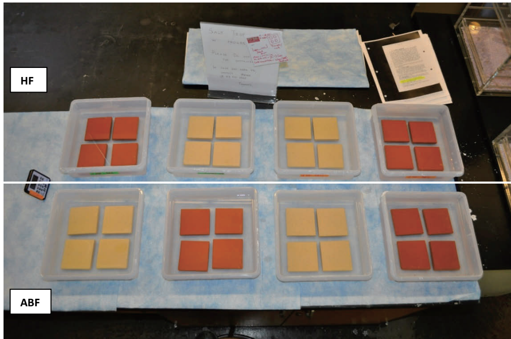
Figure 5: Two hours immersion of the samples during salt test
