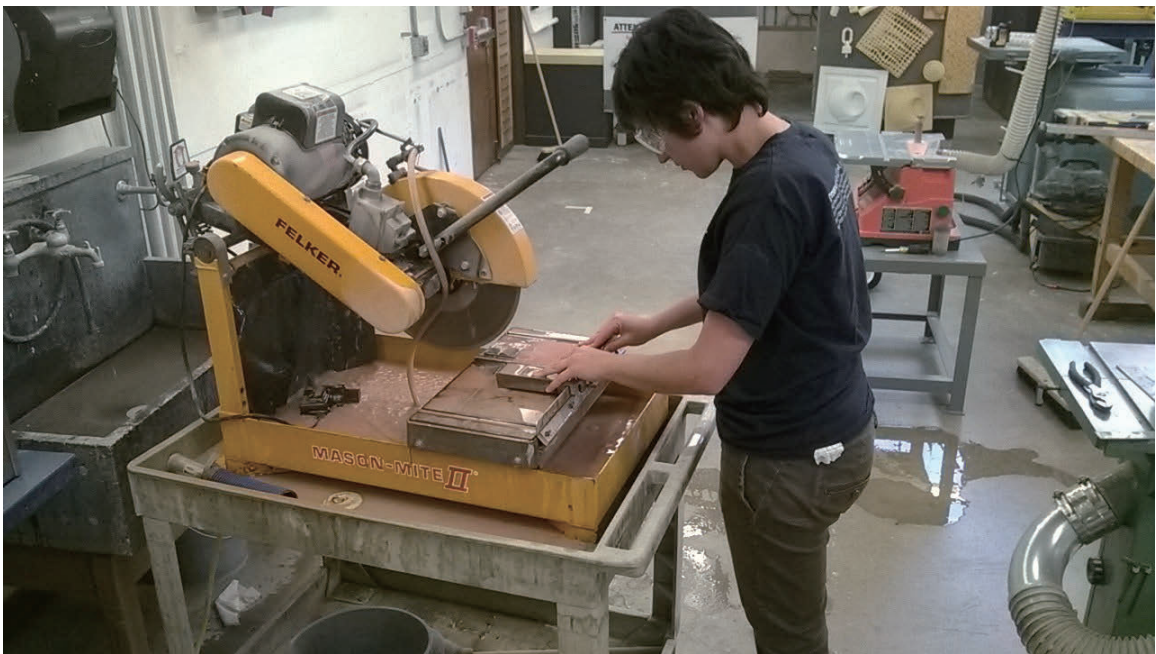
Figure 12: Cutting samples in the fab lab
