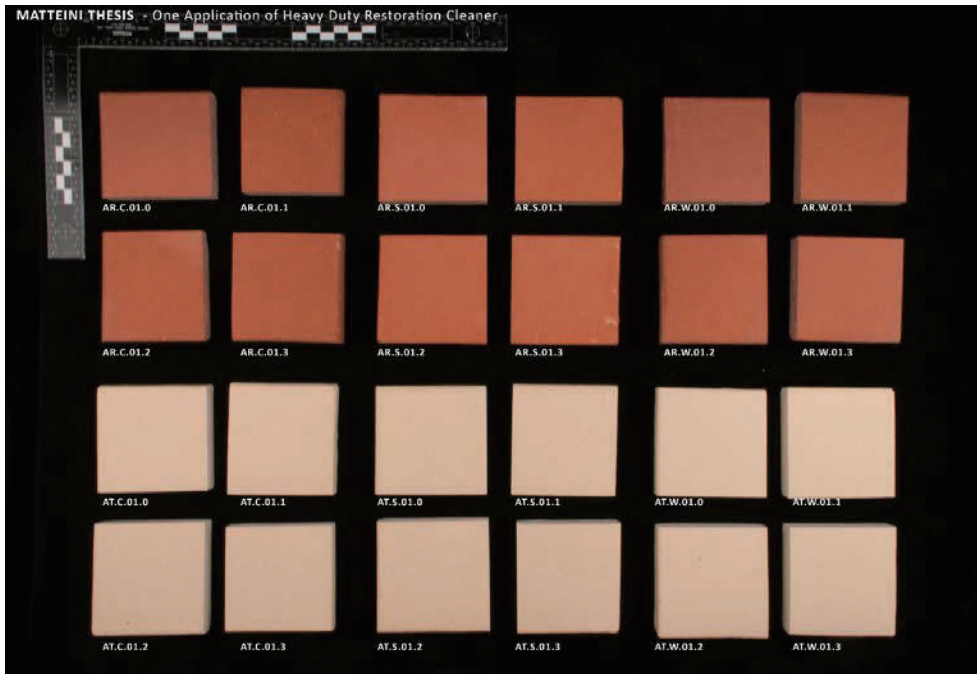
Figure 14: Sample set treated with one application of ProSoCo Heavy Duty Restoration Cleaner
