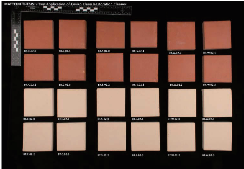
Figure 17: Sample set treated with two applications of ProSoCo Enviro Klean Restoration Cleaner
