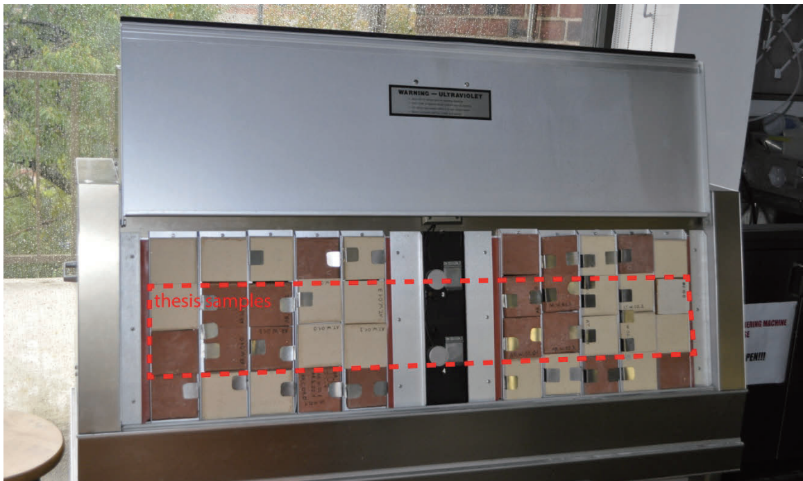
Figure 7: Samples were only displayed in the center area for a better exposure inside the weatherometer
