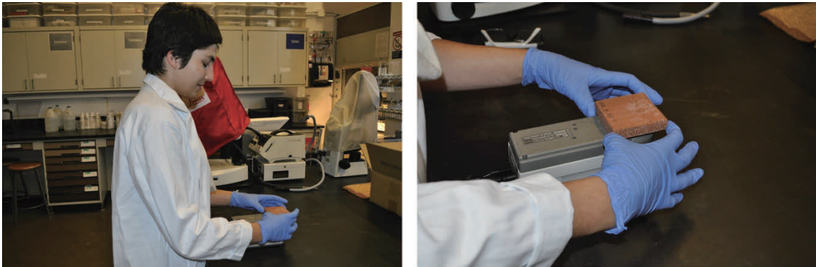
Figure 23: Irene completing a reading on a red tile with the Minolta Spectrophotometer.
