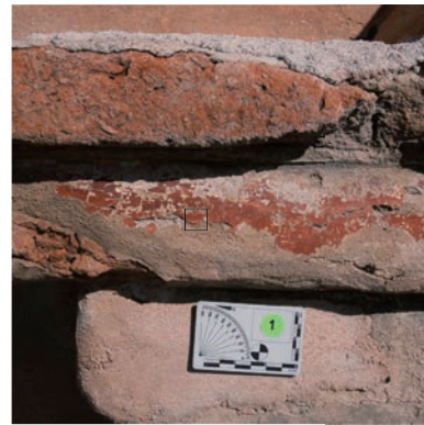
TUMA_1 Red on white undercoat, fired brick substrate
