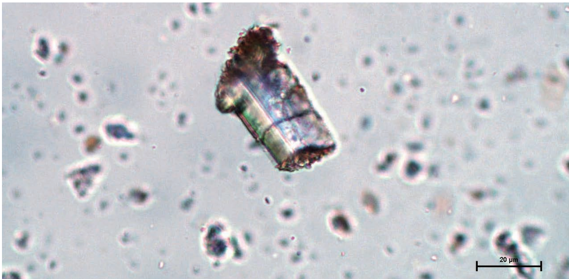
Two particles both from TUMA_12 at 400x magnification showing what appears to be quartz crystals covered in a red globular pigment – this is consistent with standards shown in Pigment Compendium
