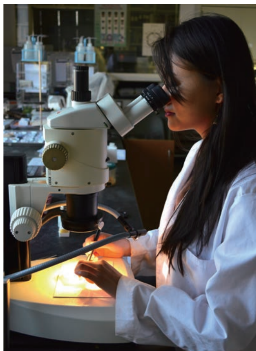
Figure 10.1: Scraping pigment particles under stereomicroscope
