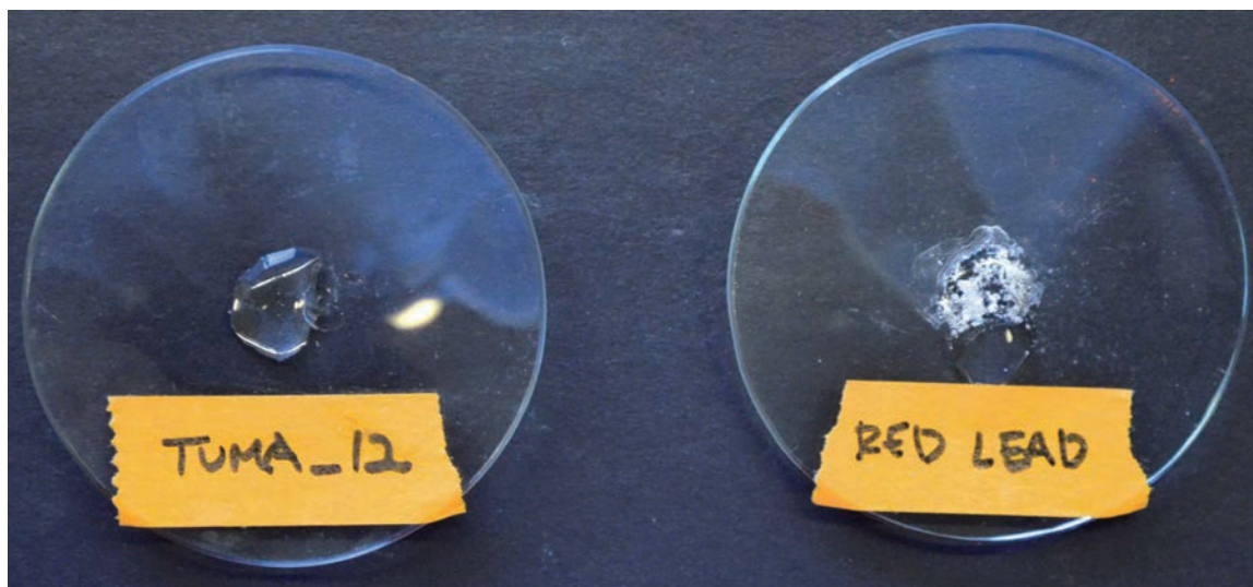
Figure 9.9: Standard samples of red lead tested alongside sample from TUMA_12 after treatment with hydrochloric acid.
