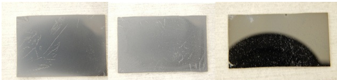
25 nm thick SiO 2 on Si wafer
