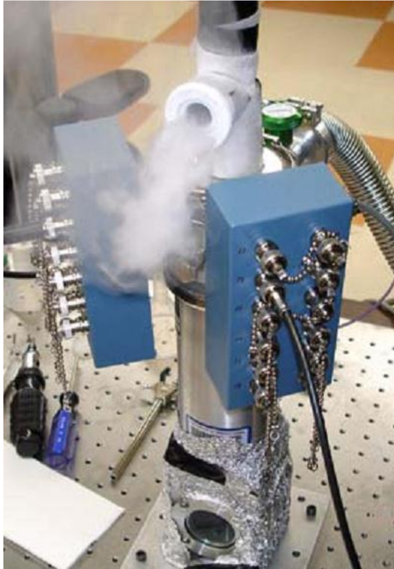
Figure 3.5.1. Cryostat in operation, with BNC breakout boxes and illumination window.
