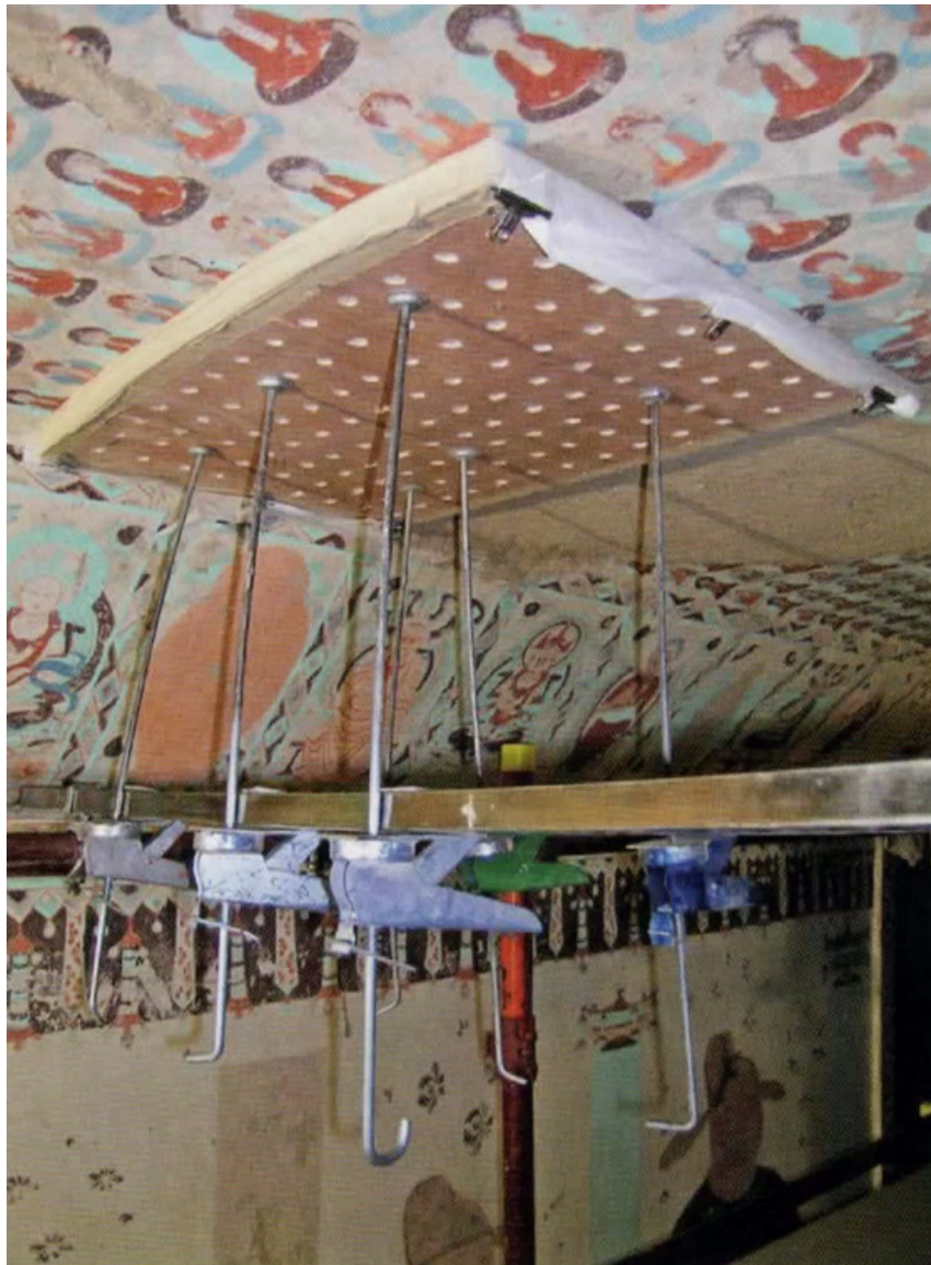
Figure 54. Custom press in cave 85 of the Mogao grottoes. Source: Stephen Rickerby et. Al. Los Angeles: The Getty Conservation Institute, 2010.
