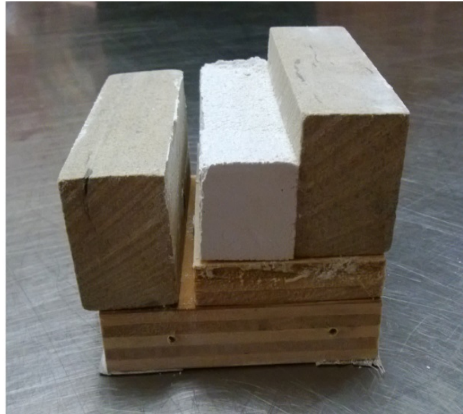
Figure 39. Plane of breakage in shear bond strength samples during curing process.
