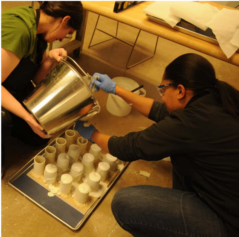
Figure 30. Pouring the grout.
