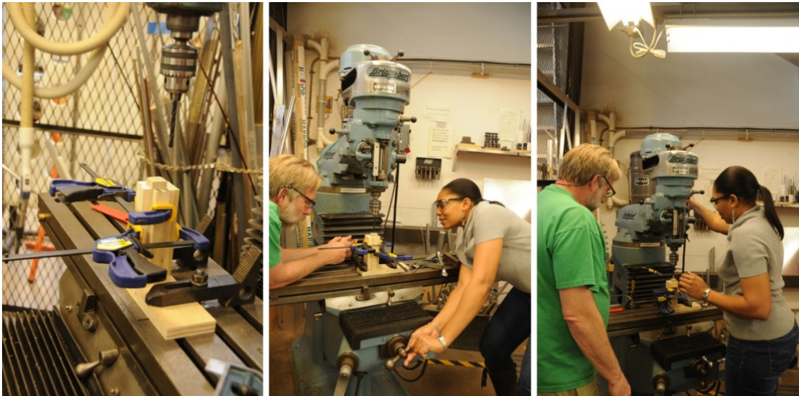
Figure 19. Peck drilling the stone on the vertical mill.
