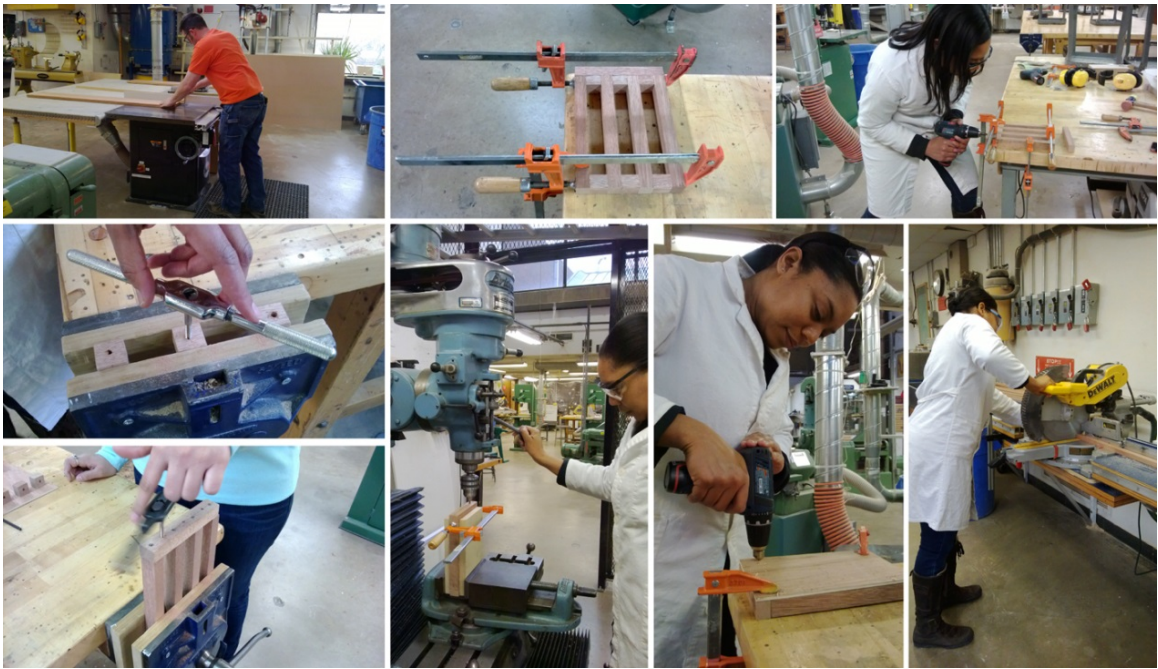
Figure 24. Preparation of molds for thermal expansion test.
