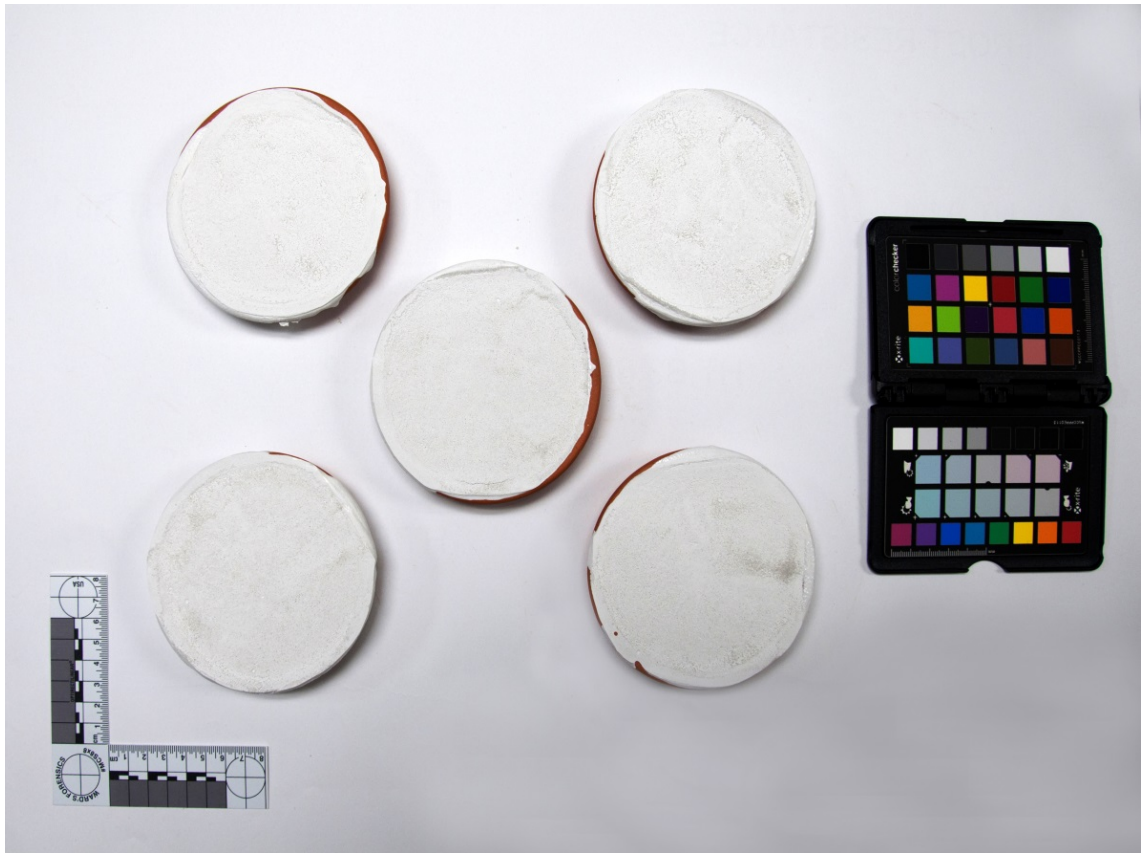
Figure 37. Photograph of visual shrinkage test samples after 28 days of curing.
