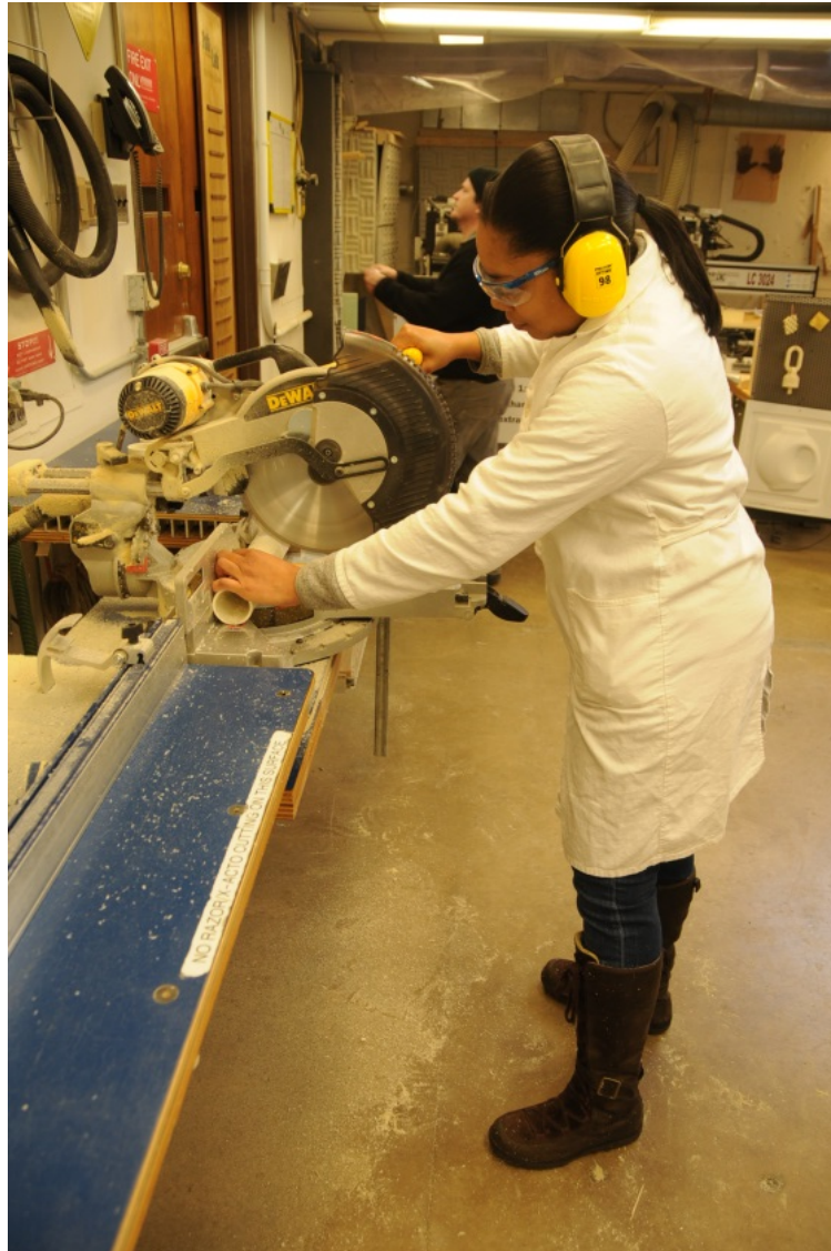
Figure 23. Cutting PVC pipe for splitting tensile strength molds with chop saw
