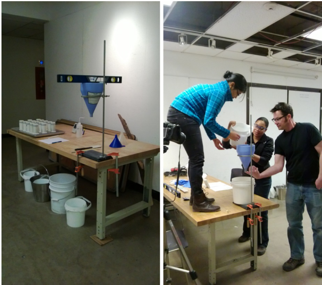
Figure 32. Leveling flow cone and performing flow test.
