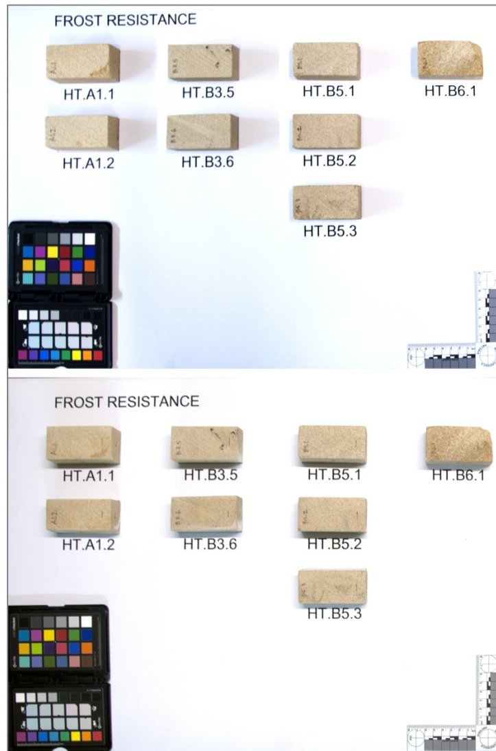
Figure 18. Samples prepared for frost resistance test prior to treatment(top) and after Fungosil Antihygro (bottom).
