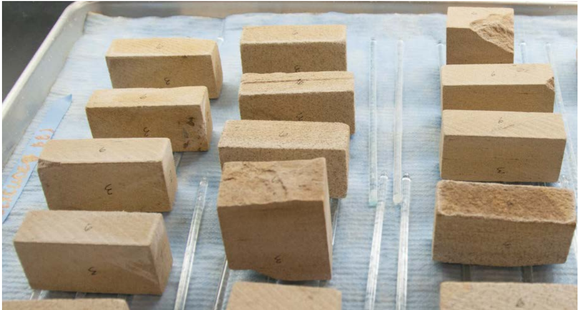
Figure 15. Formation of white residue after pre-treatment with Fungosil Antihygro.
