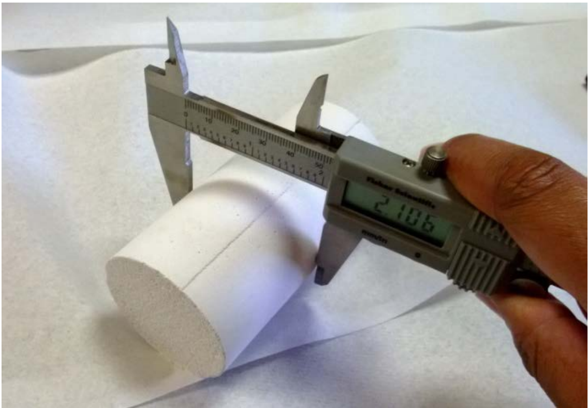
Figure 34. Measuring the diameter of the grout cylinders with digital calipers.
