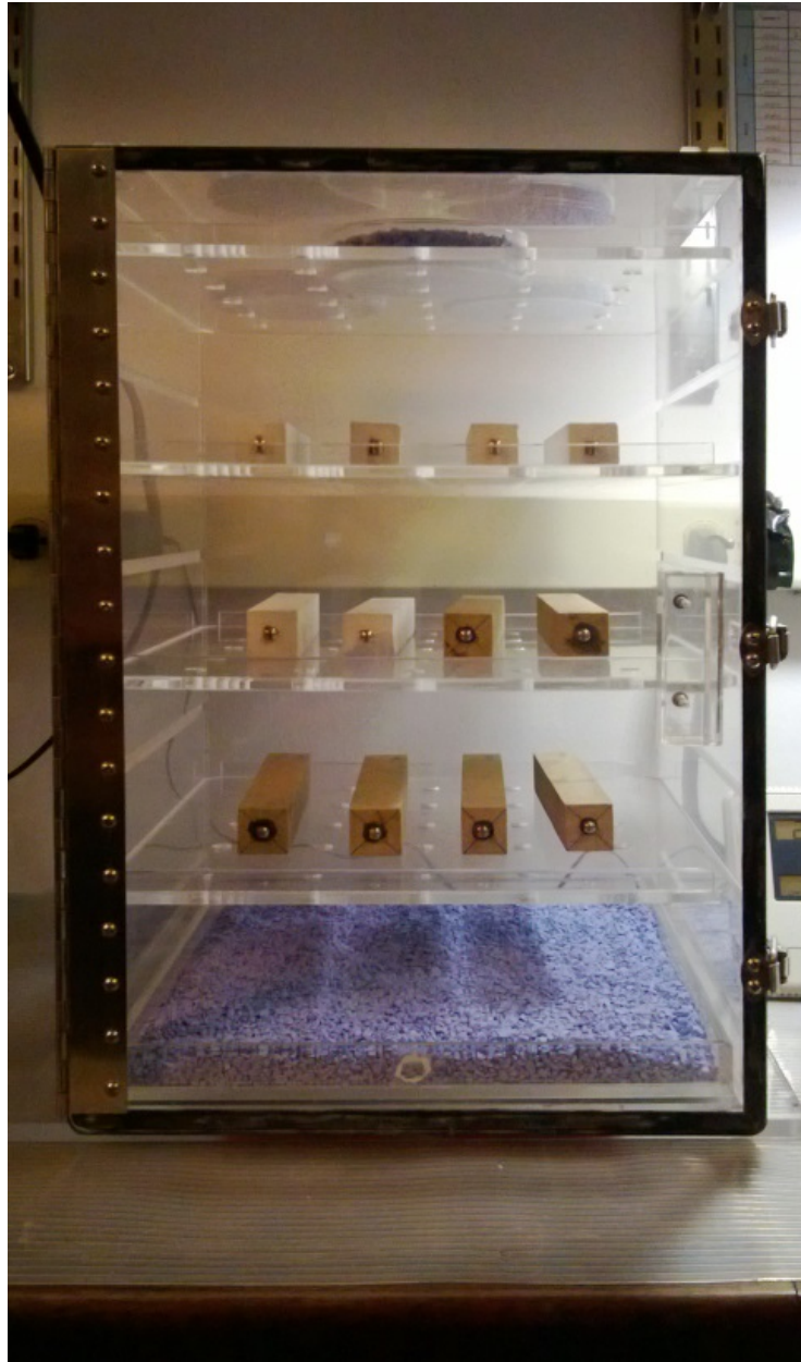
Figure 52. Grout and stone samples in desiccator.
