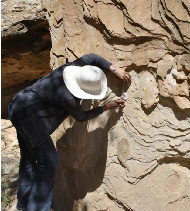
Figure 11. Preparations for RILEM water absorption test. Sources: Laura Lacombe and Milot Berisha, 2013.
