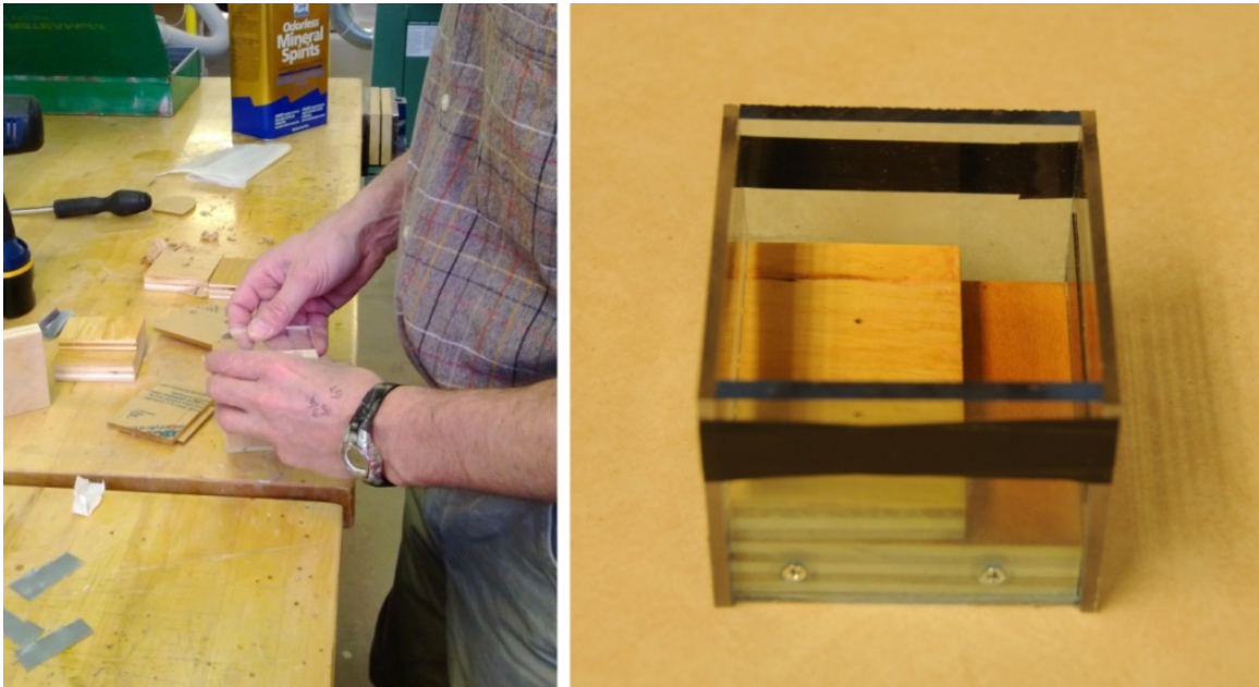
Figure 25. Construction of the shear bond strength molds
