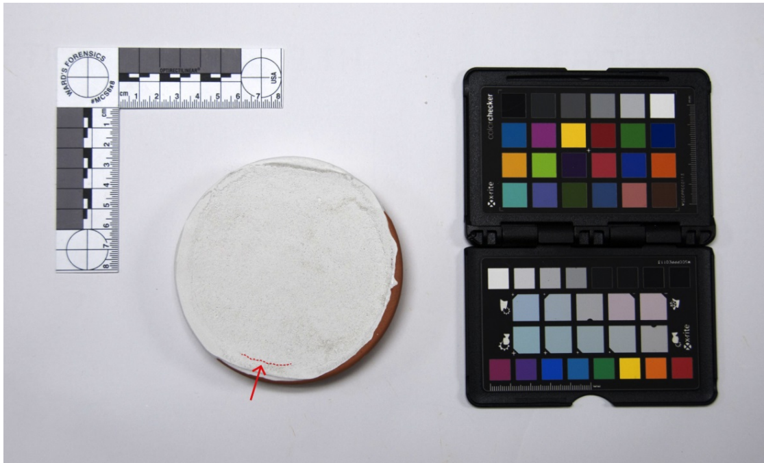
Figure 38. Detail photograph of cracking along the perimeter of the sample.
