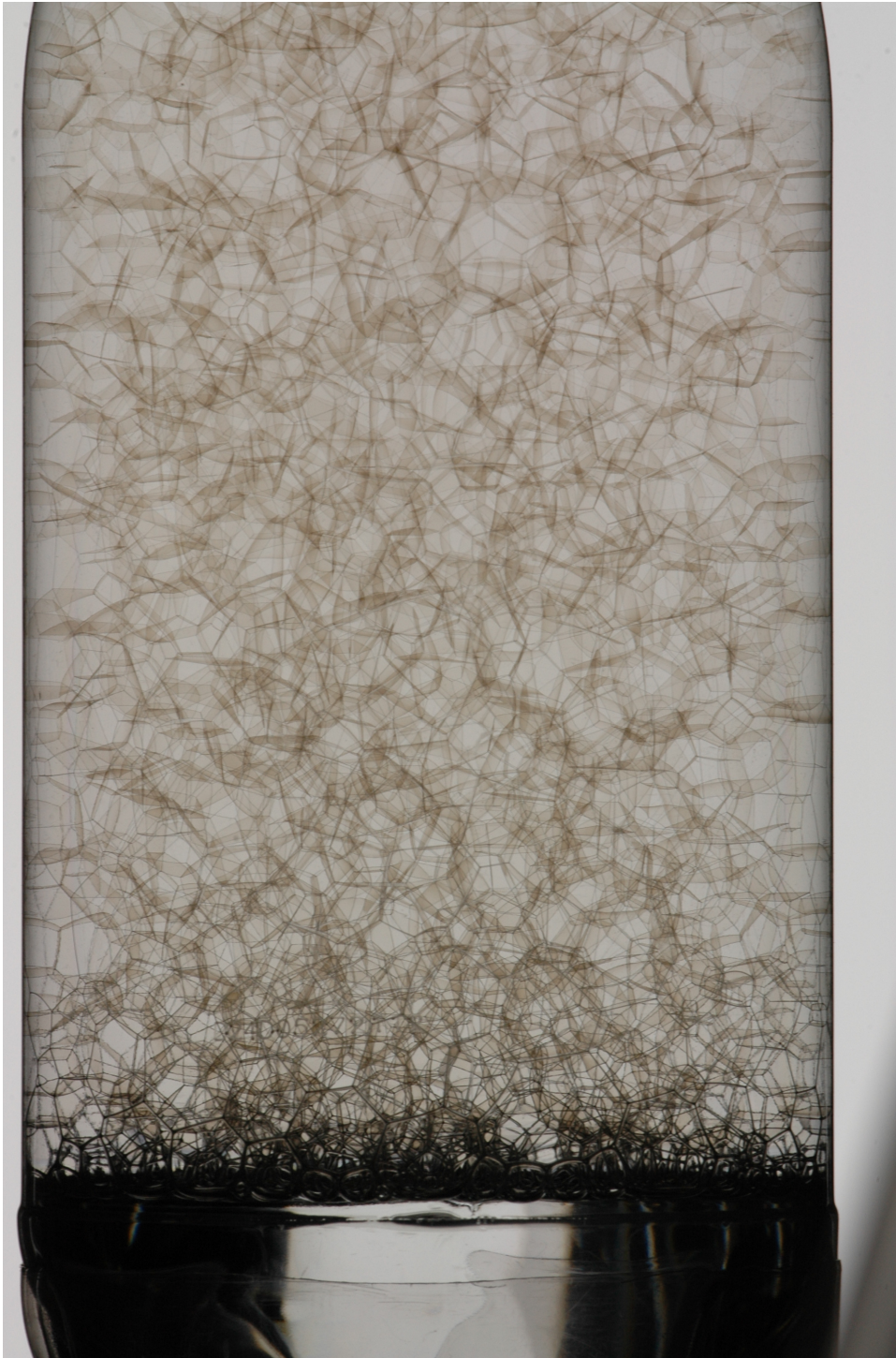
Figure 6.2: Sample photograph of bottle filled with foam sample. 720 similar photographs taken at regular angle intervals are used in the reconstruction of the foam sample slices.
