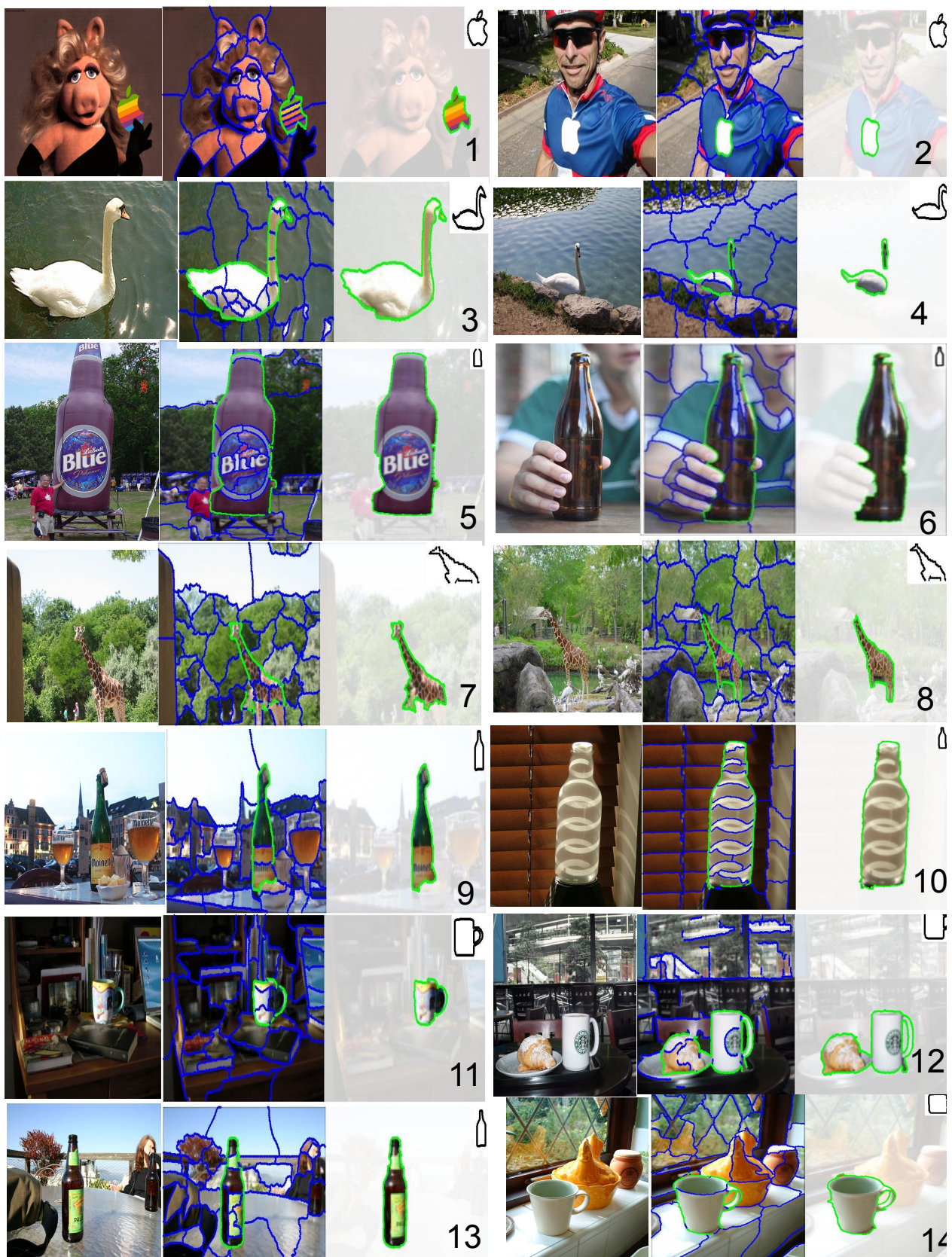
Fig. 17 Example detection on ETZ Shape dataset. For each example, we show on the left side the input image; in the middle selected superpixel boundaries; and on the right the selected object mask.
