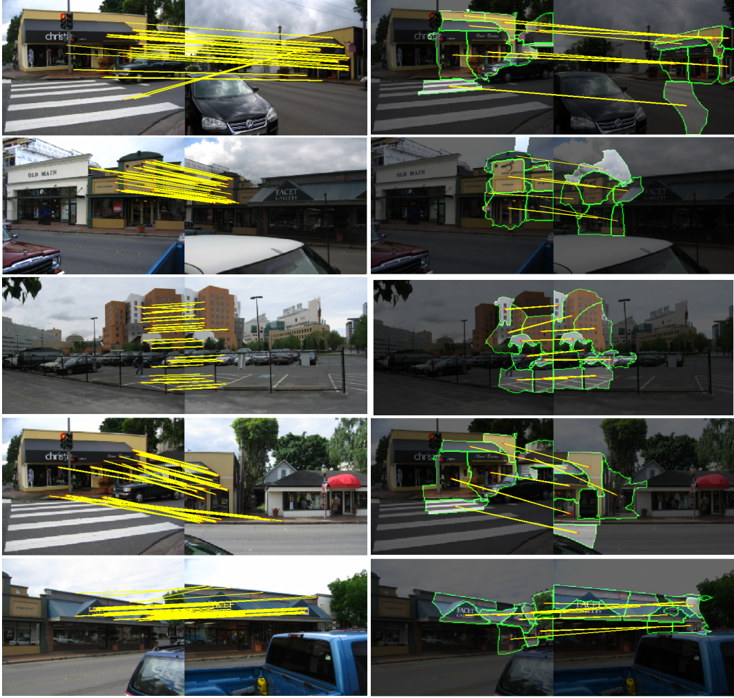
Figure 6. Matching results for manually selected pairs of images from [9]. For each pair, the top 30 matches are displayed in the left column, while the top 6 matched segments according to the match score function are presented in the right column.
