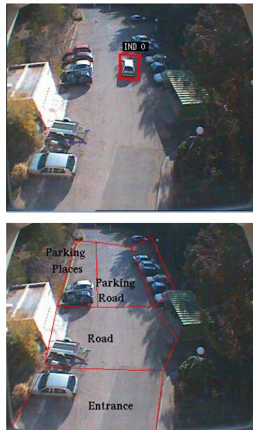
Figure 1. (a) Visualization of the event 'vehicle on the parking road'. (b) Manually defined zones in the scene.
