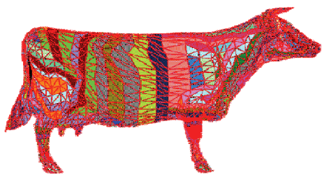
FIGURE 5: Applying stripification to a cow mesh [50]. Different colors represent different triangle strips. ( http://www.cosy.sbg.ac.at/~held/projects/strips/strips.html )
