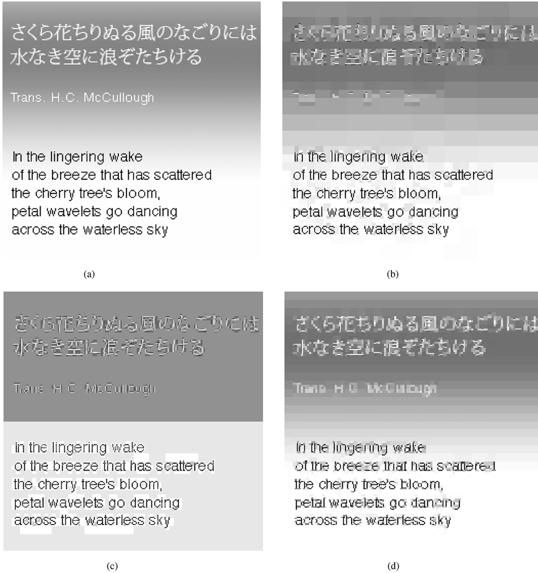
Fig. 2. Representing an image with embedded text using the optimal strategy that minimizes the \ell_2 error, and our greedy approximation algorithm under the \ell_\infty and \ell_1 error measures. The Haar wavelet is used in all three representations, and the number of retained coefficients is B = 3840 (a) The original image. (b) Output of the optimal \ell_2 algorithm (which retains the largest B wavelet coefficients). (c) Output of our greedy algorithm under \ell_\infty . (d) Output of our greedy algorithm under \ell_1 .
