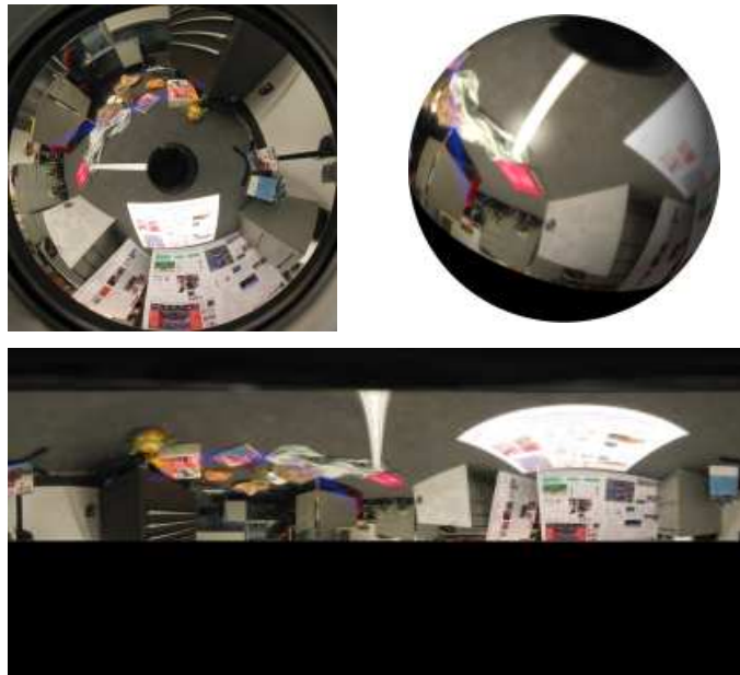
Figure 8: Top Left: a parabolic catadioptric image. Bottom: the corresponding image on a uniformly sampled spherical grid. As the parabolic mirror images only a little more than half the sphere, you can see the lower portion of the spherical image contains no information. Top Right: the spherical image as it would appear on the surface of the sphere.
