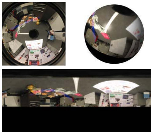
Figure 3. Top Left: a parabolic catadioptric image. Bottom: the corresponding spherical image on a uniformly sampled polar grid. Top Right: the spherical image as it would appear on the surface of the sphere
