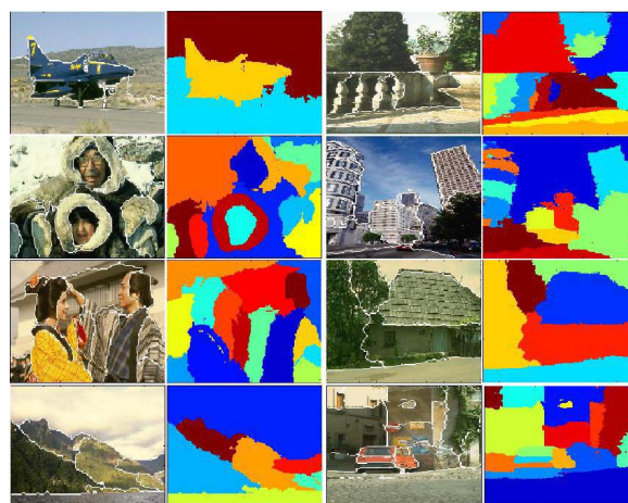
Figure 12: Multiscale Ncut prevents breaking large uniform image regions into smaller parts due to its efficient use of long range graph connections.
