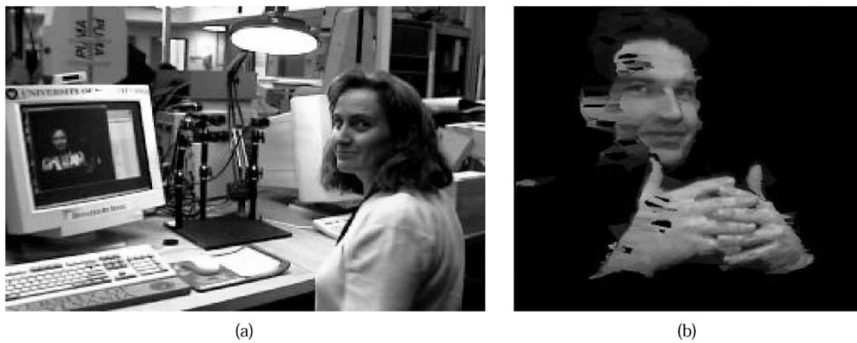
Fig. 1. (a) First networked prototype used shutter glasses and a monitor for stereoscopic viewing. (b) Binocular stereo depth maps were triangulated and rendered.
