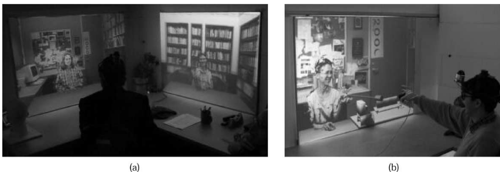
Fig. 3. Working prototypes from May and October 2000. (a) In May, the University of Pennsylvania and advanced network and services each transmitted five simultaneous trinocular depth streams to the University of North Carolina Chapel Hill. (b) In October, 3-D interaction and synthetic objects were added to the collaborative environment.
