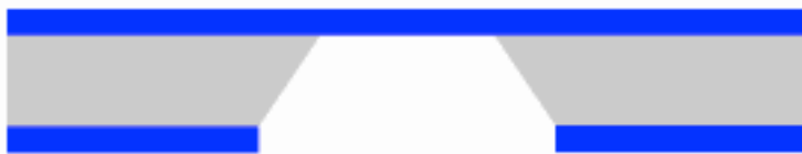
Figure 2: \text{SiN} membrane on Si chip, left by KOH wet etch. Not drawn to scale, though the angle is correct.
