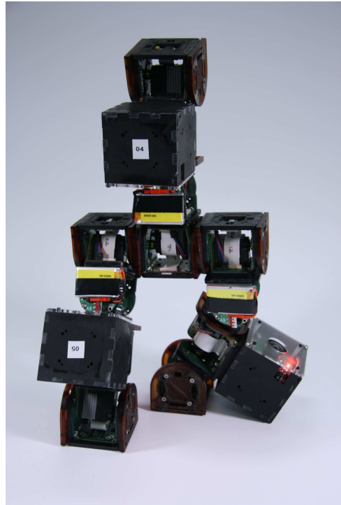
Figure 2.1: One CKBot module and an assembly of 15 modules that form the self-reassembling robot. Photos courtesy Jimmy Sastra.
