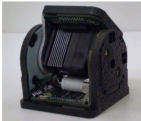
Figure 2.1: One CKBot module and an assembly of 15 modules that form the self-reassembling robot. Photos courtesy Jimmy Sastra.
