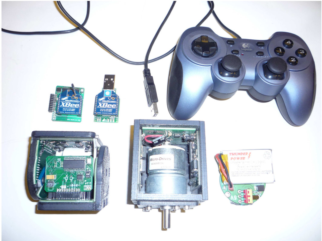
Figure 2.5: Various CKBot peripheral devices. Clockwise from top left: ZigBee wireless system, joystick, Lithium-Polymer battery board, DC Leg Module, and Submodule controller inside an L7 module.
