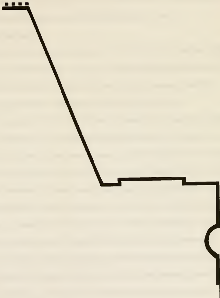
FIGURE 3.3.12 Plaster cornice profile in the Southeast Parlor, probably dating from ceiling replacement in 1885. Drawing by author, actual size.
