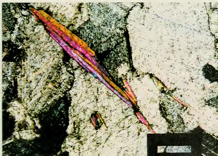
Figure 2. Thin Section of Sample I, crossed polars, 100X. Micaceous inclusion, interlocking calcite grains.
