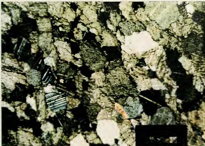
Figure 1. Thin Section of Sample I, crossed polars, 25X. Note twinning and tight interlocking of calcite grains.
