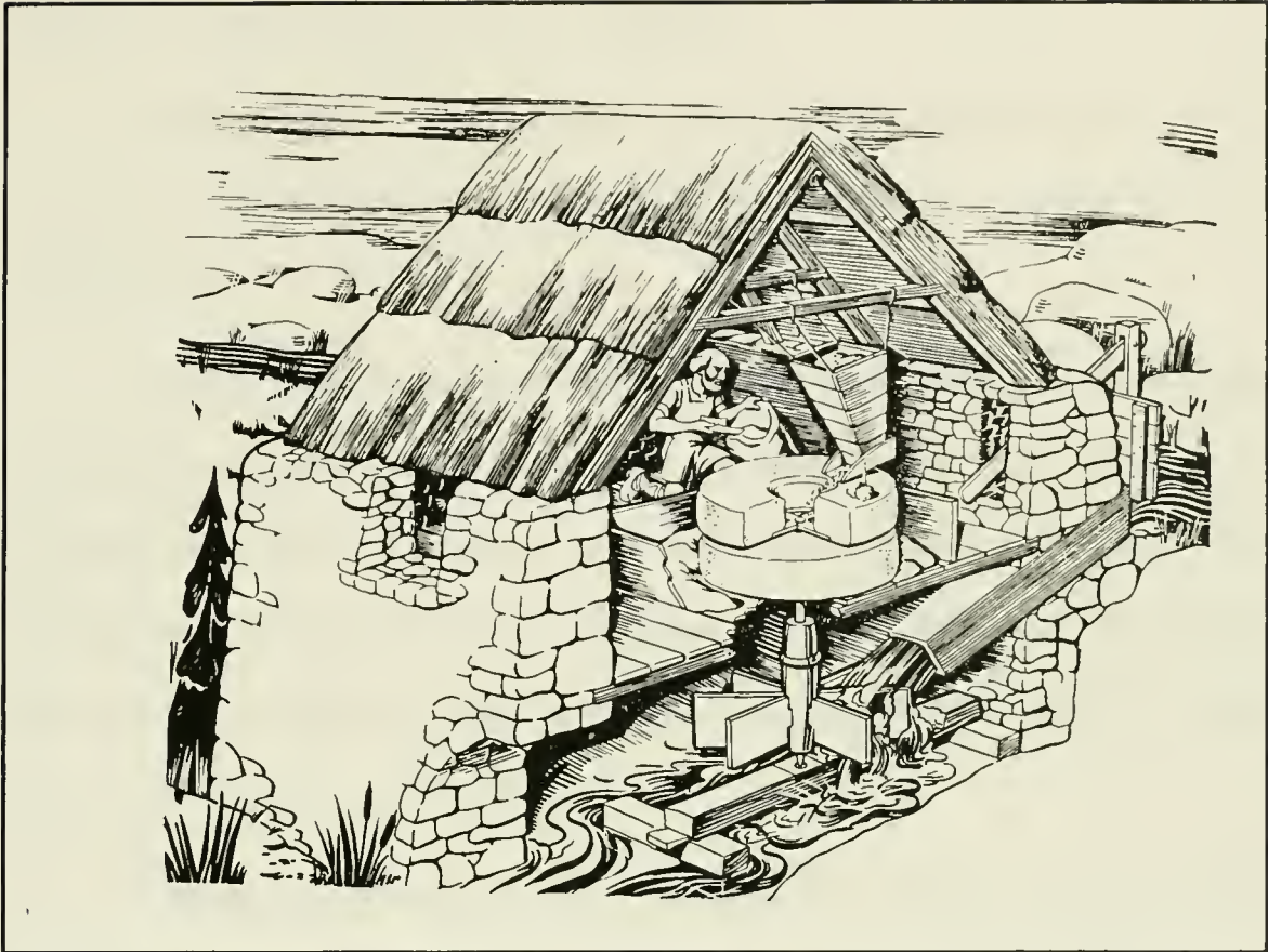
Fig. 5 Norse-type direct-drive mill, Scotland (Storck pg. 98)
