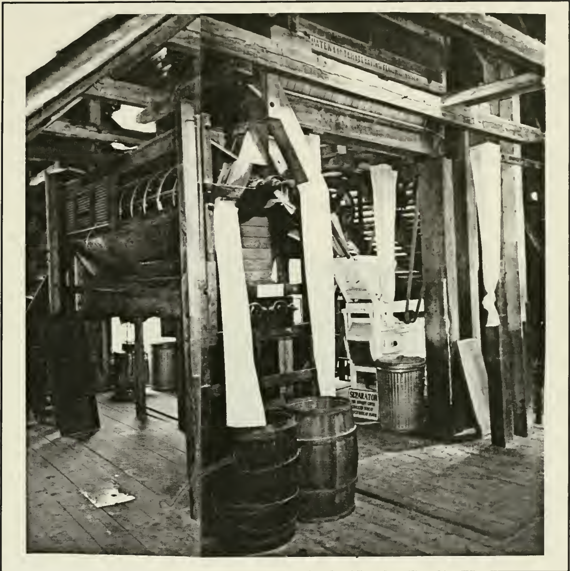
Fig 23 The Bolting Machinery
