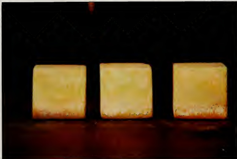
Figure V.12 Back sides of non-nummulitic samples L4, L5, and L6 (from left to right) after impregnation with saturated solution of NaCl and following drying.
