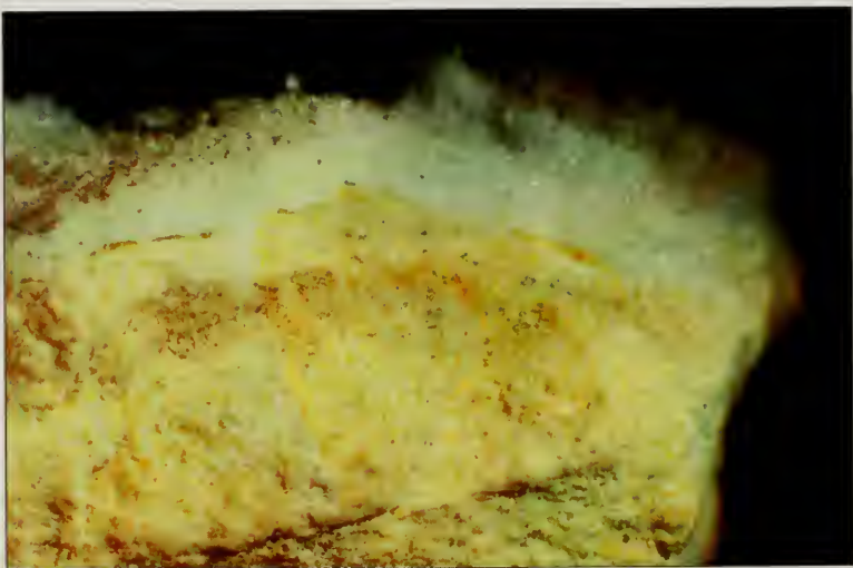
Figure IV.11 Layered salt crust on limestone from a surface flake ( U sample ). Total magnification \times 2.5 .
