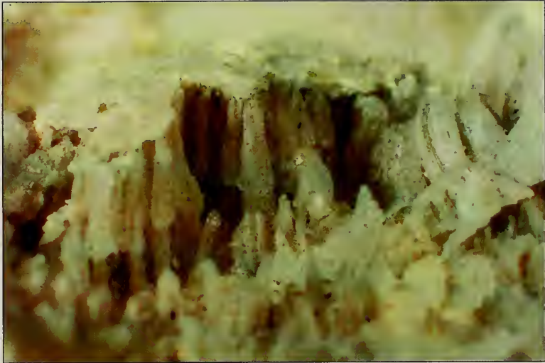
Figure IV.14 Detail of typical layered sinter forms of parallel prisms and needle of calcite arranged in layers (U sample). Total magnification \times 3.125 .
