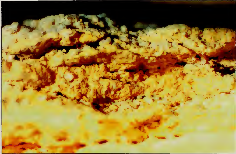
Figure IV.16 Flaking and delamination of the stone surface caused by salt crystallization. Sample 9, possibly Comit  repair stone from a recently excavated area. Total magnification \times 5 .
