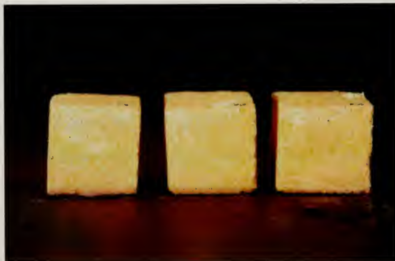
Figure V.13 Back sides of nummulitic samples F4, F5, and F6 (from left to right) after impregnation with saturated solution of NaCl and following drying.
