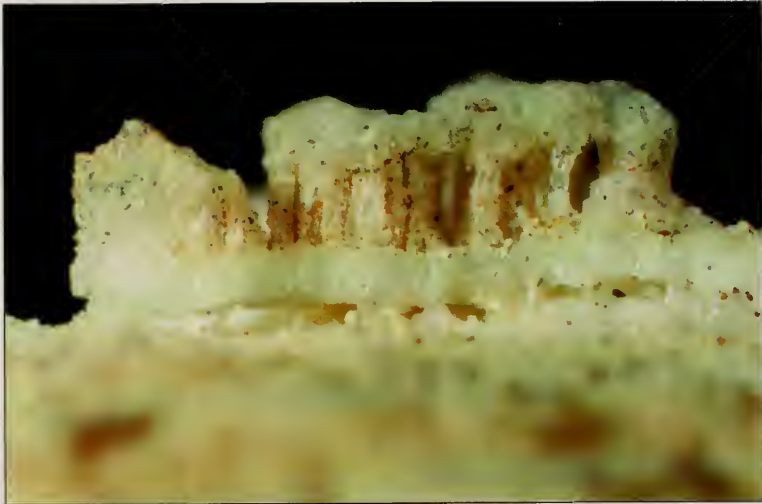
Figure IV.12 Detail of parallel columnar calcite crystals elongated perpendicularly to the layers, in previous sample (U sample). Total magnification \times 6.25 .
