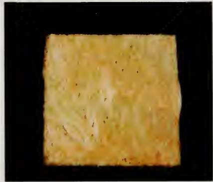
Figure V.14 Back side of non-nummulitic samples L4 after impregnation with saturated solution of NaCl and following drying showing preferential salt crystallization pattern.
