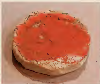
Fig 5.20 Sample from Tomb #275, Gray Group stucco showing salts from the stucco forming at the interface of brick skin during the capillary absorption test.
