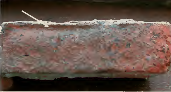
Fig. 5.2 A hand made brick evidenced by the lip formed when brick was removed from its mold before being fully dry.
