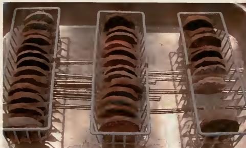
Fig. 5.19 Stucco discs racked in water for capillary absorption test.
