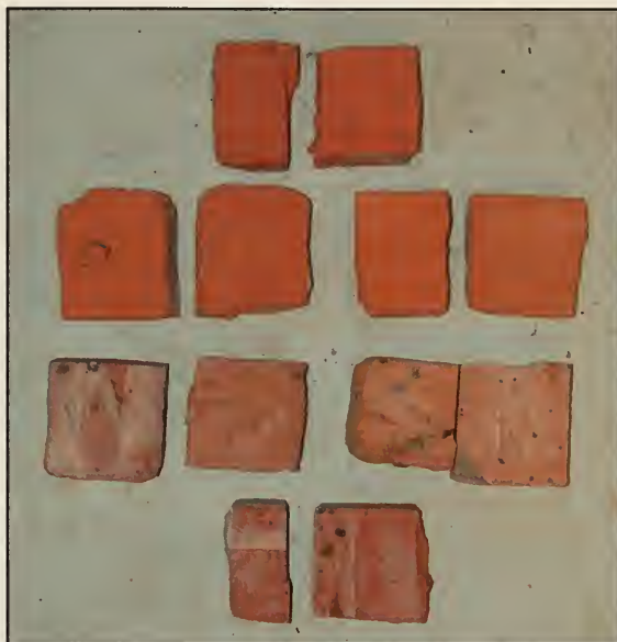
Fig. 5.5 Examples of brick samples. The top six samples are River brick which tend to be red to reddish orange. The bottom six samples are Lake brick, which are tan to pink and usually have spots of burnt impurities.
