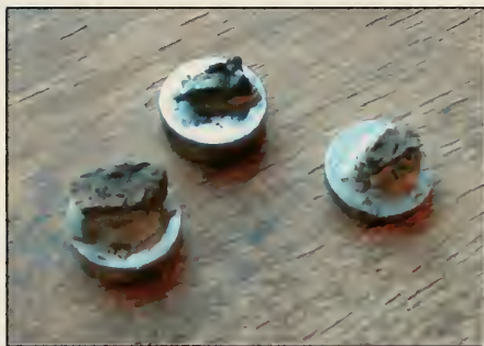
Fig. 5.43 Stucco samples mounted for SEM analysis.
