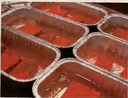
Fig. 5.11 Total immersion test on brick.
