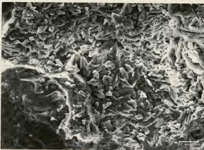
Fig. 5.50 Tomb #200, A highly magnified view of a pore with re-crystallized calcite, characterized by soft, rounded crystals, 1000 x.
