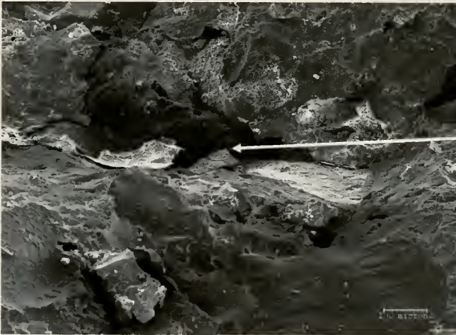
Fig. 5.48 Tomb #200, Interface between Dark Tan (top) and Gray (bottom) Stucco Layers, 100x. Note cracks and air spaces at the interface.
