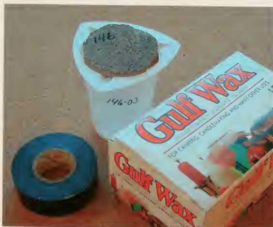
Fig. 5.14 Stucco sample preparation for WVT test.
