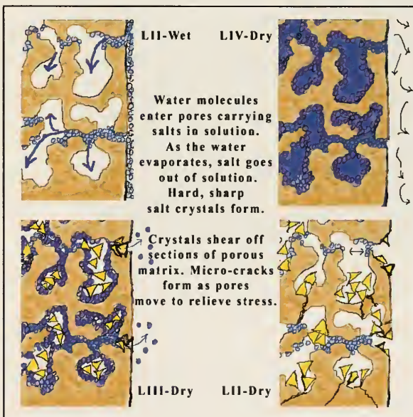
Fig. 3.14 The salt decay mechanism is a progressive mechanism, causing greater decay the more cycles the material experiences.
