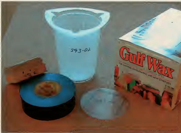
Fig. 5.15 Brick cubes for WVT test.
