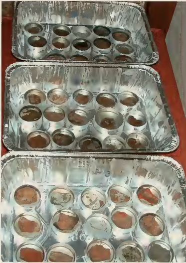
Fig. 5.6 Samples of stucco during total immersion test.
