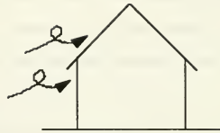
Missing Sheathing/ Shingles Upward Movement (Dynamic Load)
