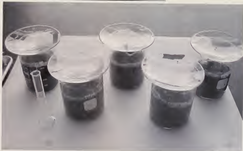
Figure 3.7. Water Retention Test in Progress
