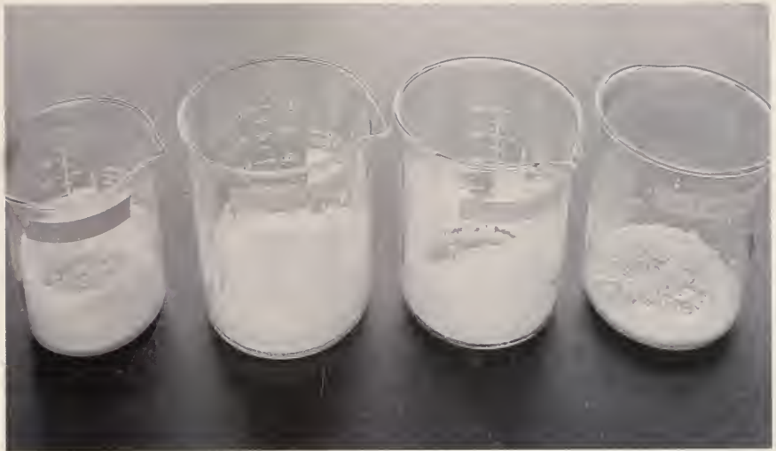
Figure 6.14. Beakers of Saturated Sodium Chloride Solution and Varying Concentrations of Triton (evaporated). From left to right: Control; 0.5% w/v Triton; 1% w/v Triton; 2% w/v Triton.
