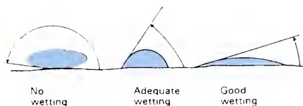
Fig. III.6 Water droplet and its contact angle. Due to the tendency of the liquid molecule to pull itself tight, it requires more energy for the droplet to increase its surface area. Water can flow without pressure and wet a surface when the contact angle is less than 90^\circ . From Dirt and Pictures Separated , 1990.
