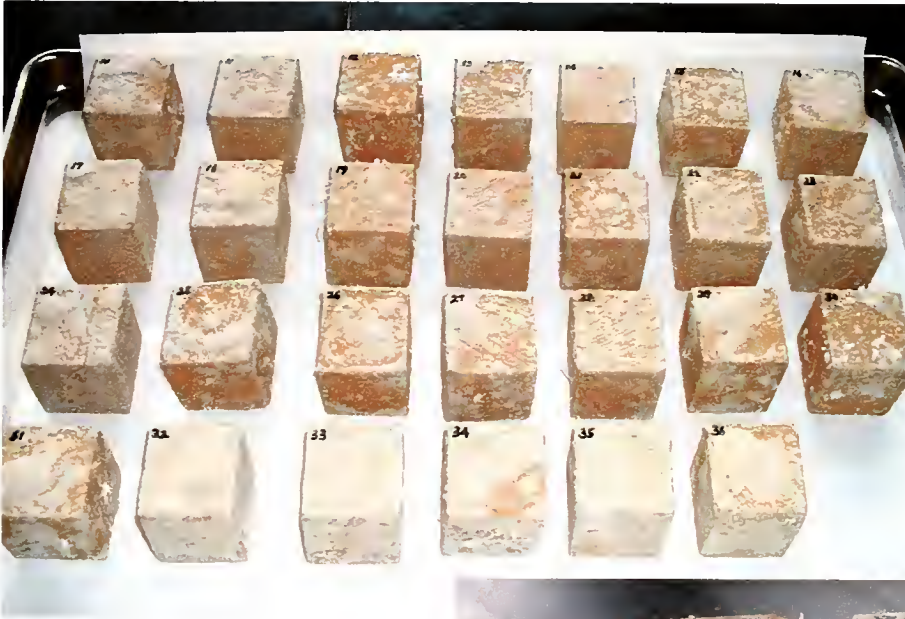
Fig. IV.3 27 samples impregnated with NaCl.
