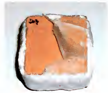
Fig. IV.6 A sample cube covered with Japanese tissue paper and paper pulp poultice.
