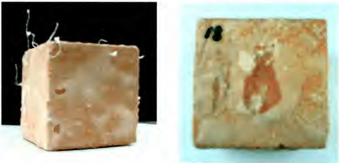
Fig. II.2 Both Egyptian limestone cubes were impregnated with NaCl. The cube on the left exhibits both whisker growth and salt crusts, whereas the sample on the right manifests only the salt crusts.
