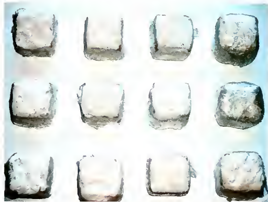
Fig. IV.7 Samples poulticed and wrapped in plastic wrap.
